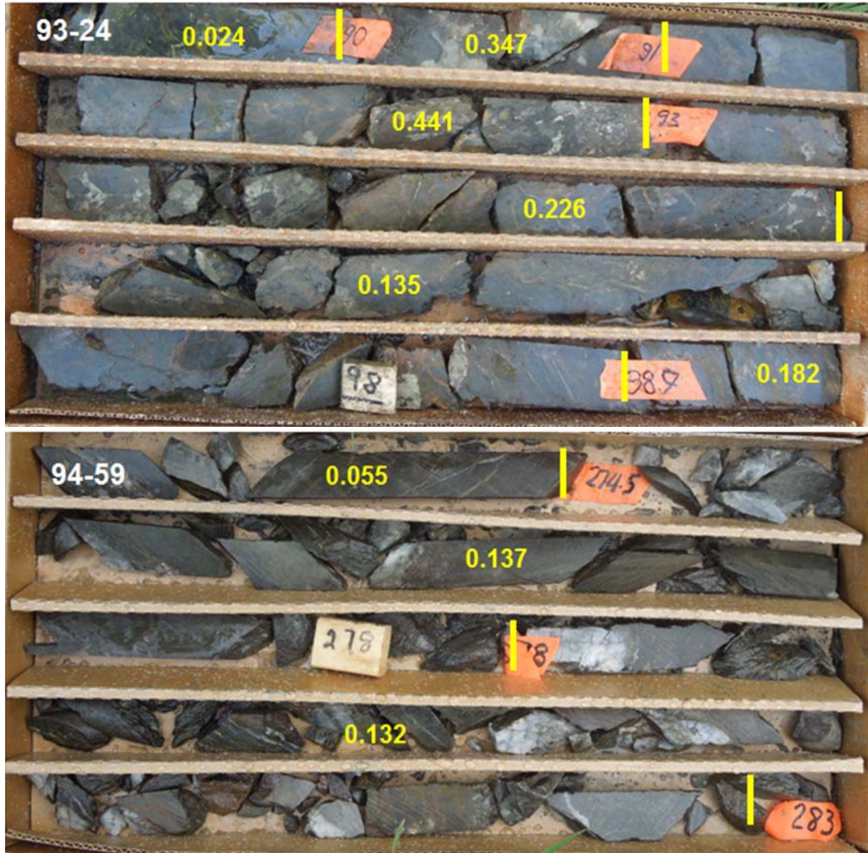
Figure 10: Energy Fuels Corporation Core Drilling from the Egyptian Deposit Area, showing Gold Grades (in ounces per ton).
