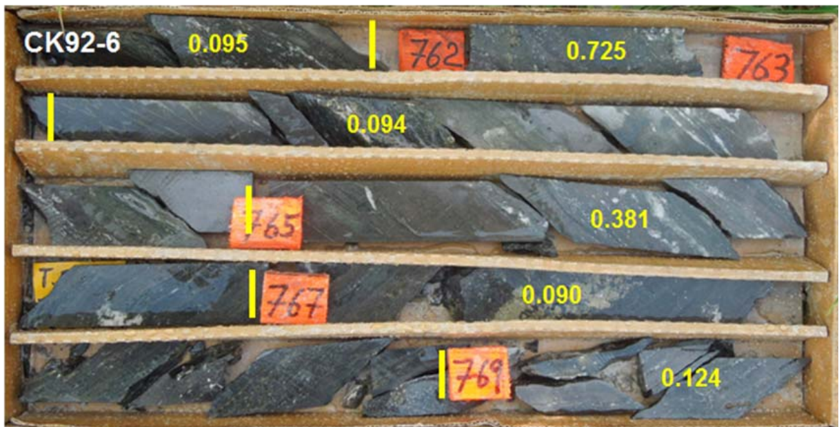
Figure 12: Cyprus Gold Core Drilling from Keystone Area (Borehole CK92_6) showing Gold Grades (in ounces per ton).
