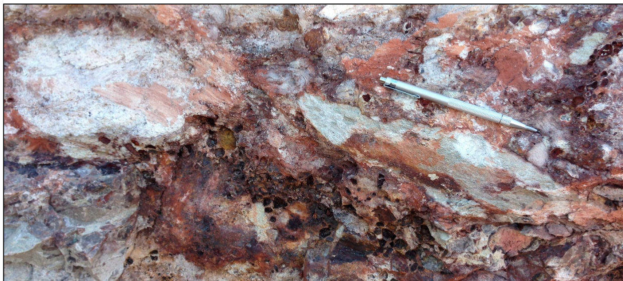
Figure 7-13: Hematitic, kaolinite altered polymictic conglomerate with remnant voids left by oxidized "buck shot" pyrite
