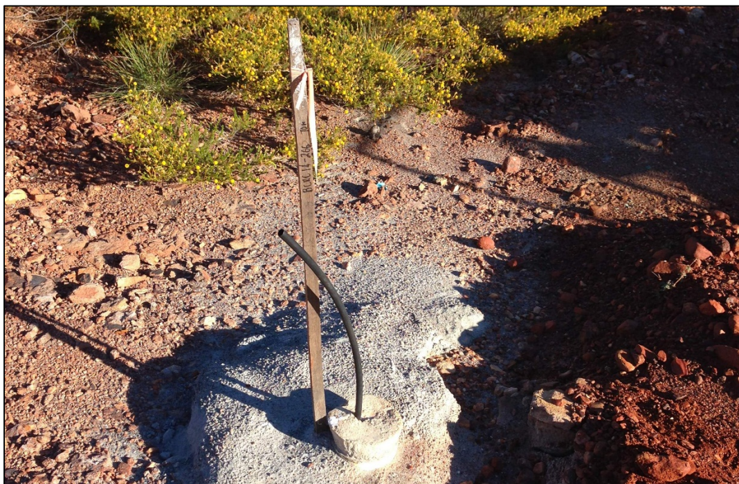
Figure 10-2: Plugged and Marked Drill Collar Monument at Beatons Creek
