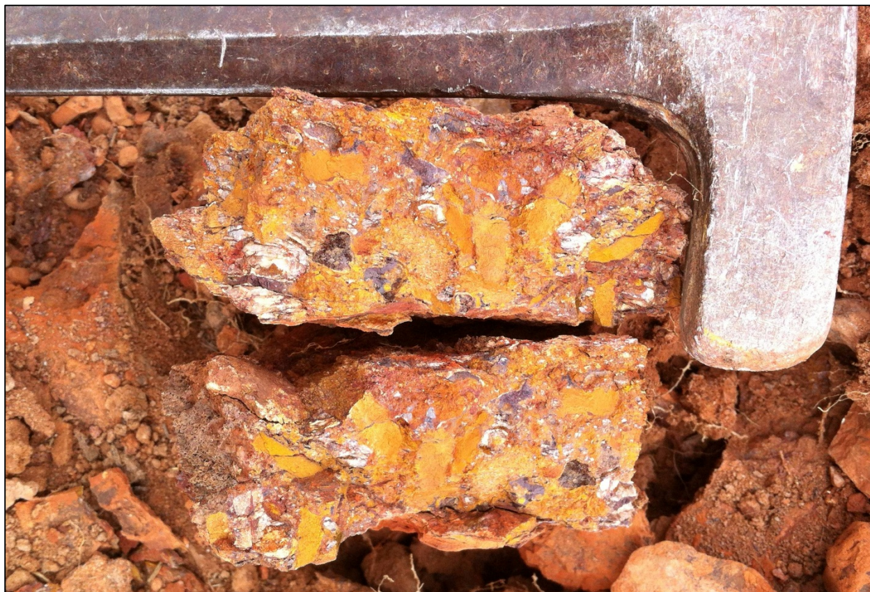
Figure 7-11: Angular yellow shale present in the matrix of armored lag type conglomerates
