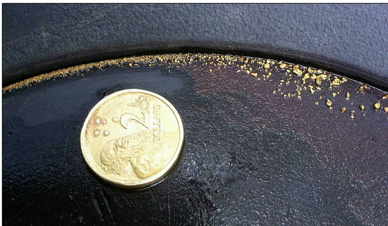
Figure 7-14: Gold panned from crushed matrix material from an armored lag type conglomerate
