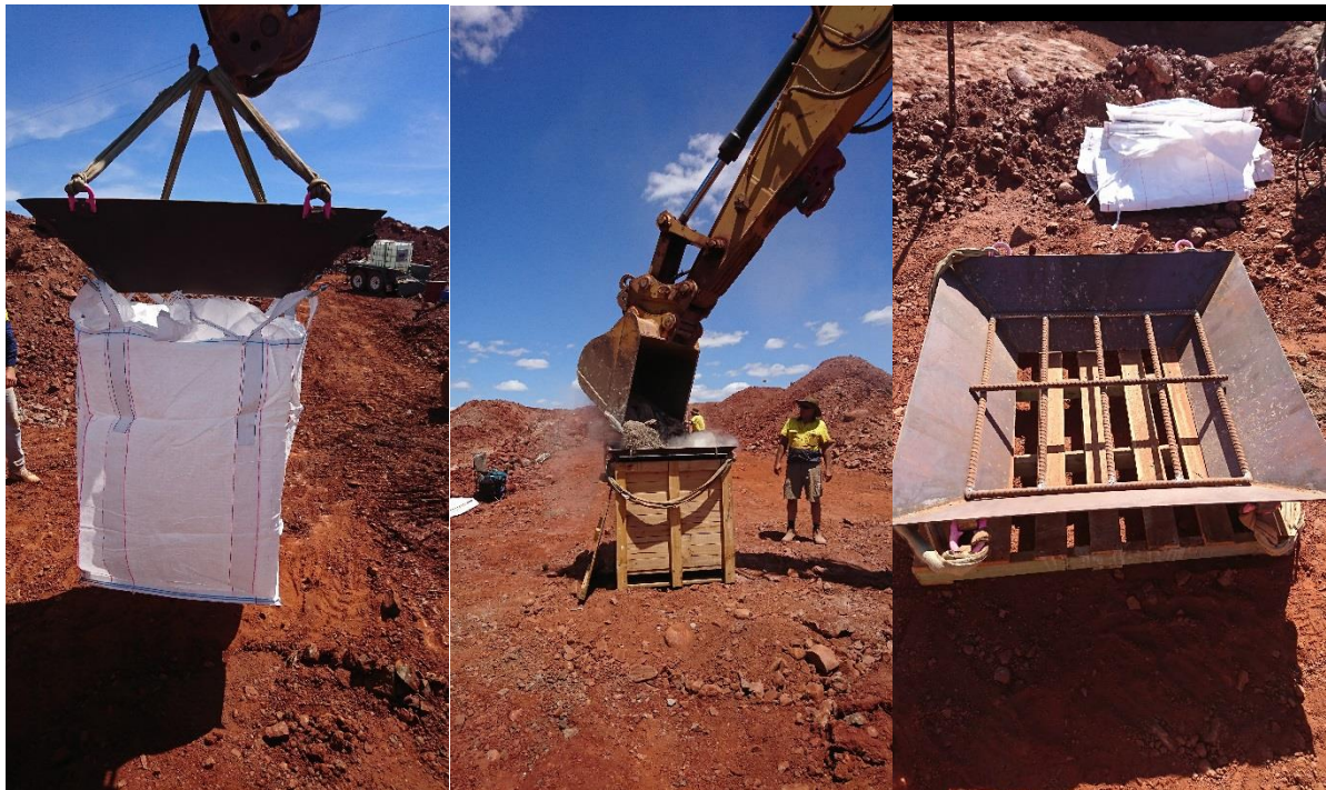
Figure 11.7 Bulka bag on hopper, about to be put into box (left). Excavator loading into hopper on box (centre). A 200 mm grizzly in hopper (right).
