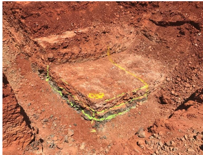
Figure 11.5 A 2 m by 2 m trench sample marked out ready for sampling at Purdy's Reward
