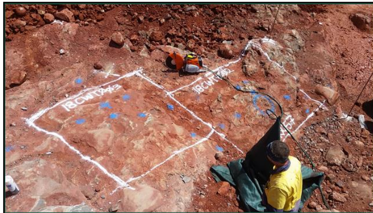
Figure 11.6 Bulk Lateral Sampling practice; Sample mark out (top), rock breaking a sample with a flyrock screen (centre), final sample location surveyed in 3D and photographed (bottom)
