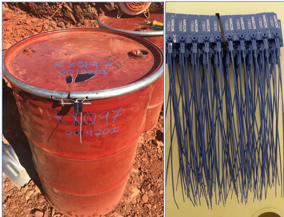
Figure 11.3 Sealed sample drum showing the locking mechanism, security seal and sample information written on the lid and side of the drum (left); examples of security tags (right)
