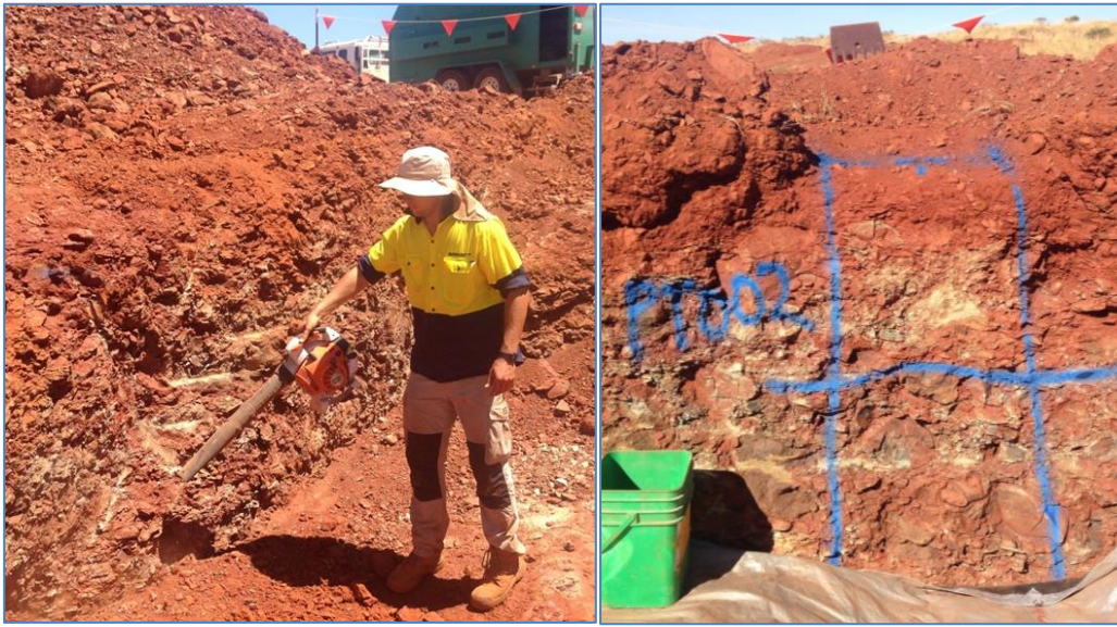
Figure 11.2 Sampling using a jack hammer (left) and transferring fines (right)
