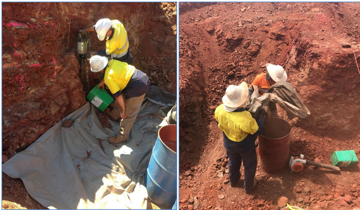
Figure 11.2 Sampling using a jack hammer (left) and transferring fines (right)
