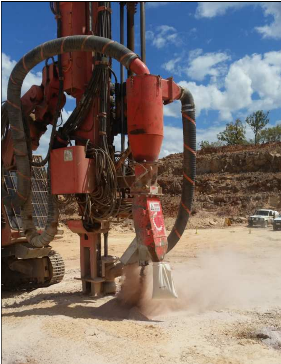
Figure 11-4. Rig-Mounted Sample Splitter
