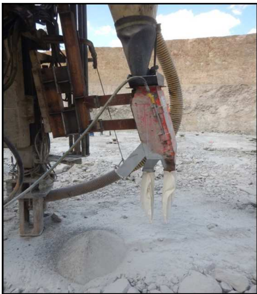
Figure 11-1. Collection of Blasthole Sample Material
