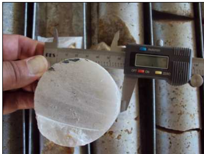
Figure 6-6. Measurement of Sample for Bulk Density Determination
