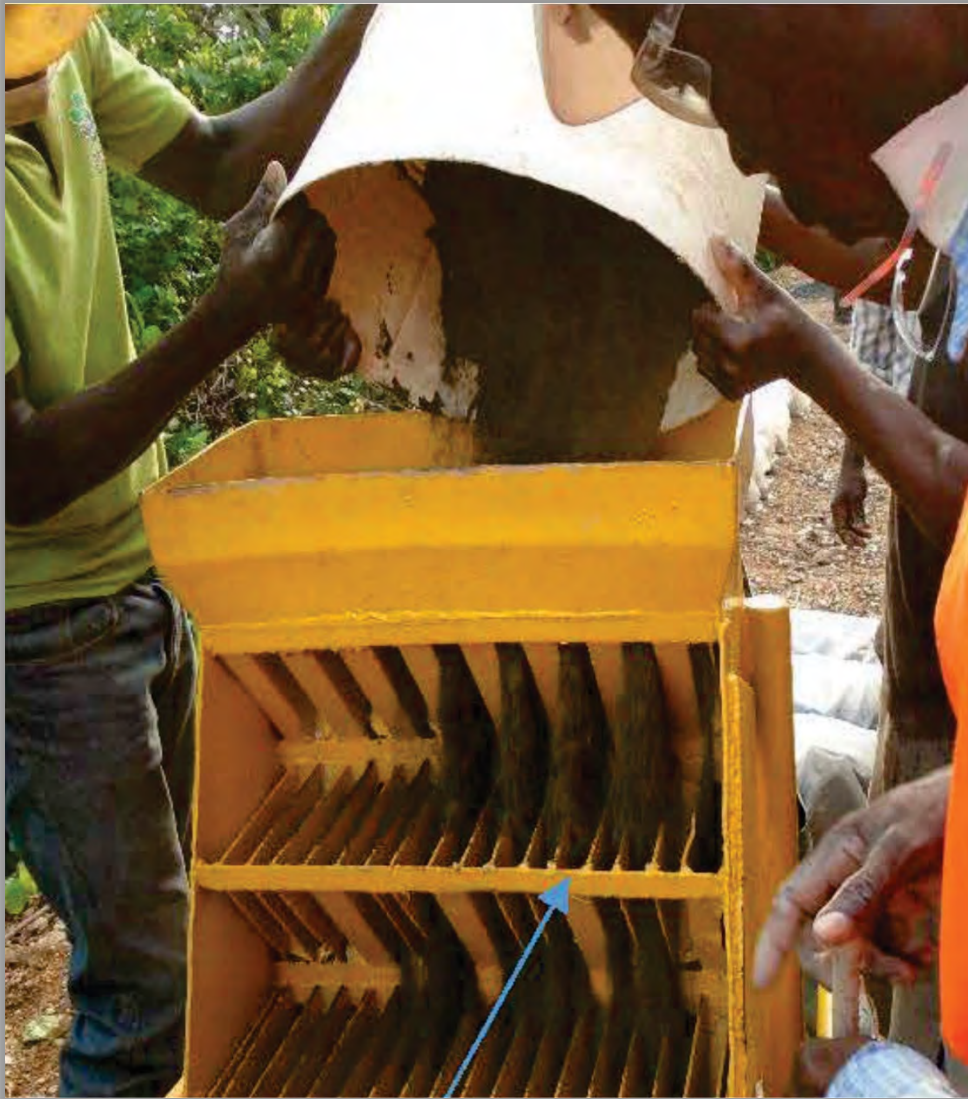
Figure 10.9 Reserve Circulation Sampling Riffle Splitter
