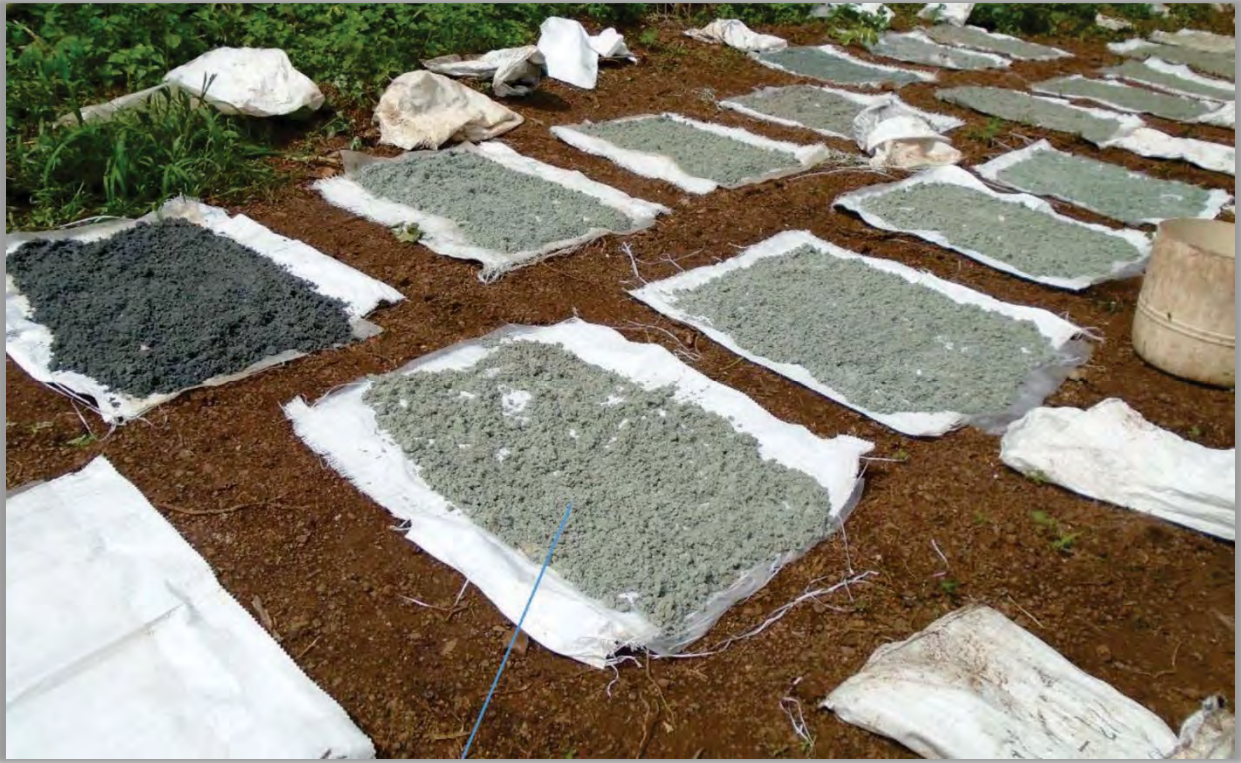
Figure 10.10 Drying Wet RC Samples
