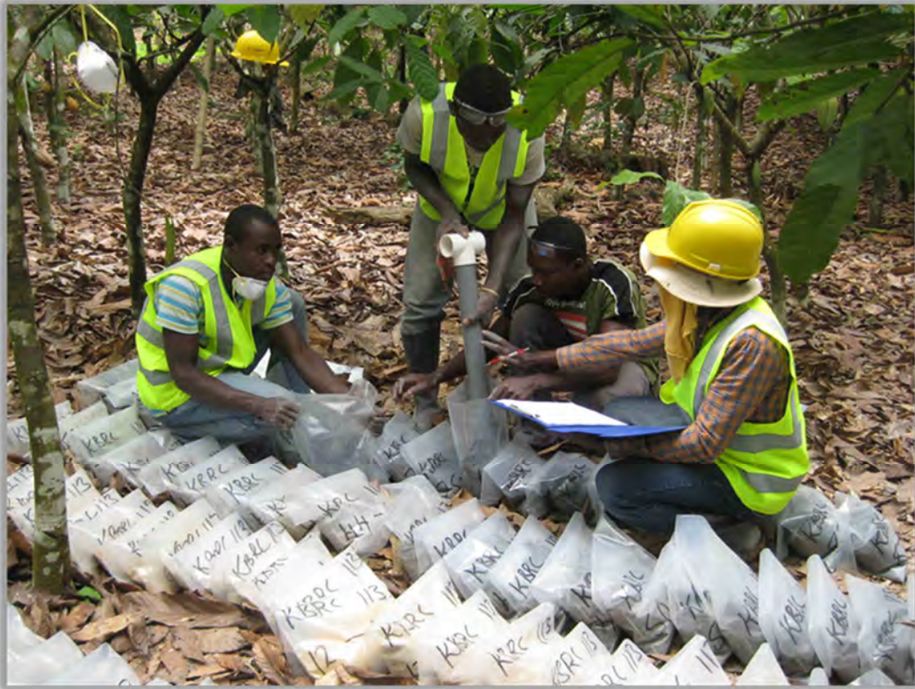
Figure 10.8 Reserve Circulation Sampling Using Tube Splitter
