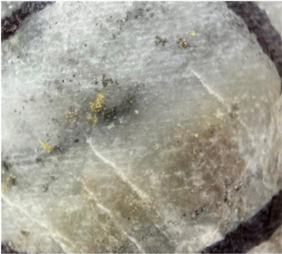
Native gold in quartz breccia at 810.5m of GS-24-181.
