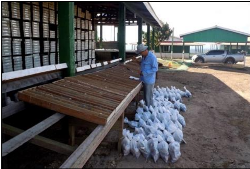
Figure 21: Drillhole samples collected and bagged in the core storage area at site
