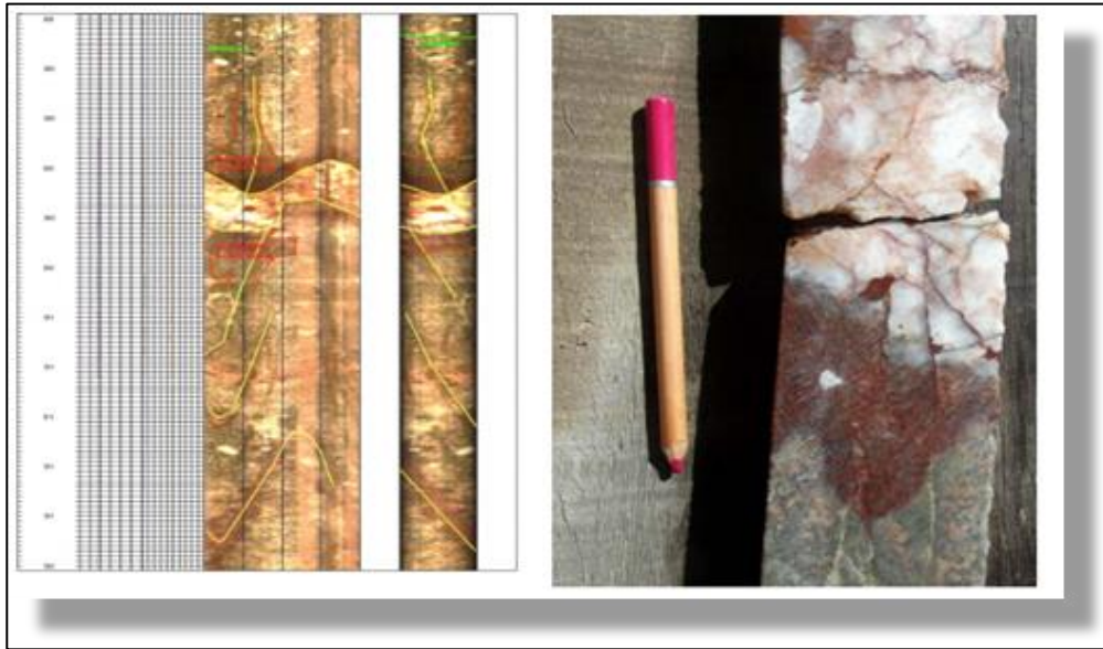
Figure 16: OTV image of a diamond hole compared with actual core from same interval
