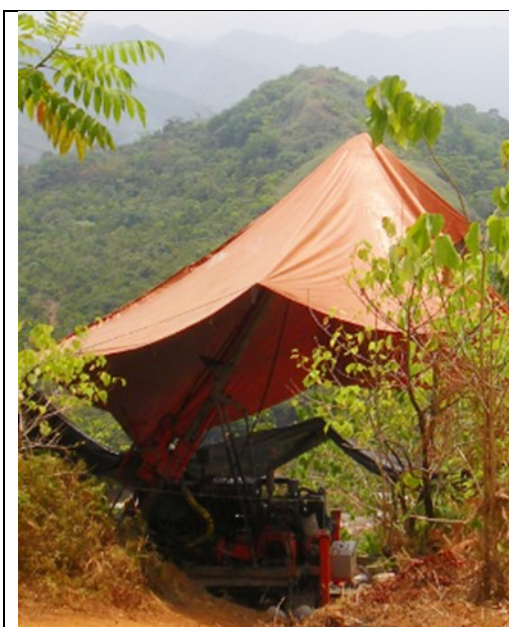
Figure 10.1. Drill Pad, ACD005, Duralite T600H diamond drill rig in operation at El Alacran.
