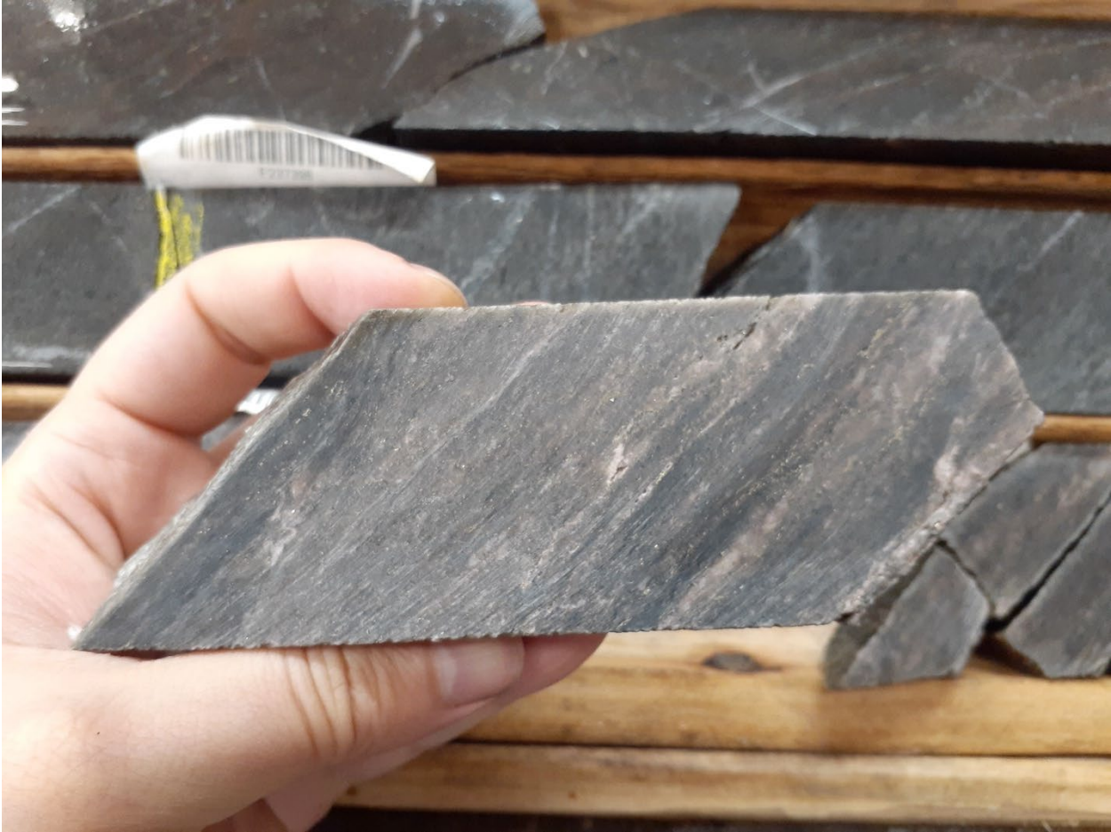
Figure 3: Drill core from 549-550m (1m @ 13.8g/t Au) in MQD-22-072 highlighting sheared, altered intrusion.
