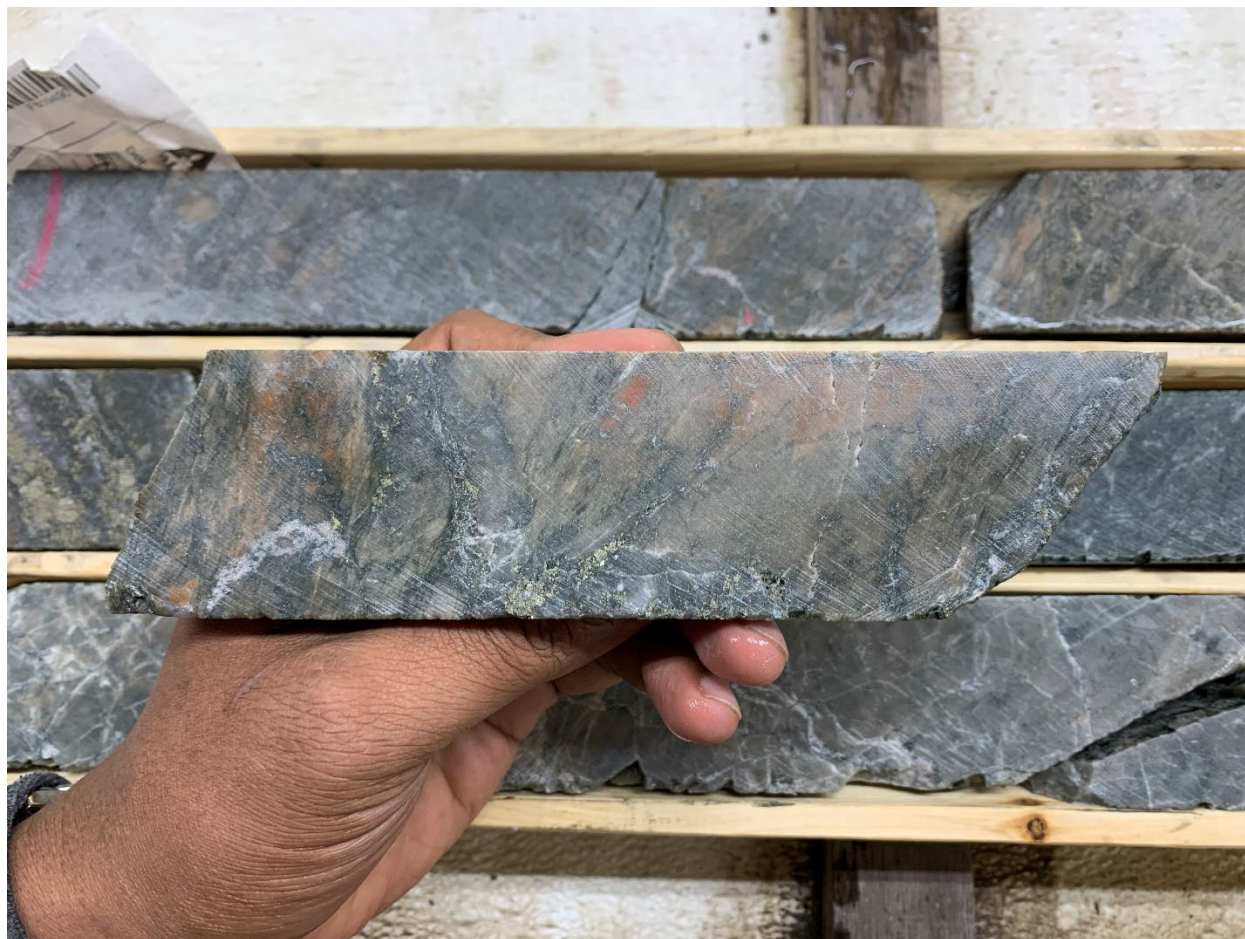
Figure 4: Drill core from 416.4 - 417.05m (0.65 m @ 36.8 g/t Au) in MMD-23-116 highlighting a pyrite + chalcopyrite mineralized quartz-carbonate vein within the sheared, altered intrusion.
