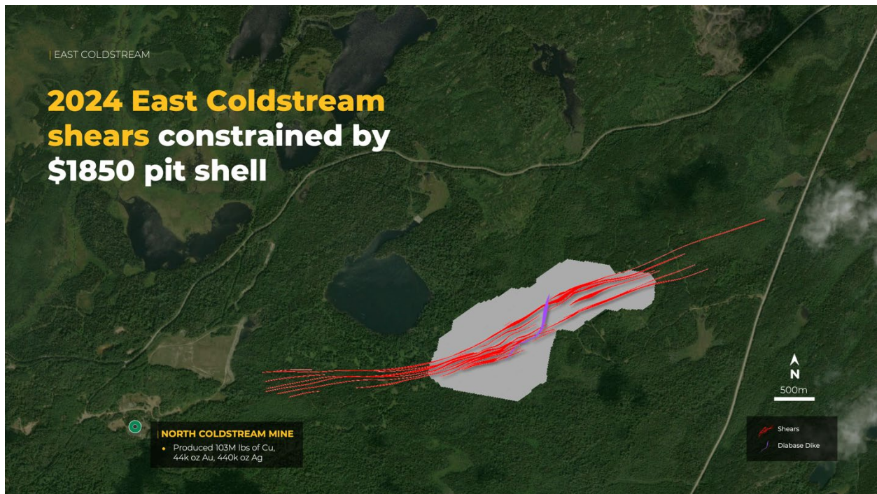
Figure 5: Plan of East Coldstream showing shears, cross-cutting diabase dike and $1,850 pit shell
