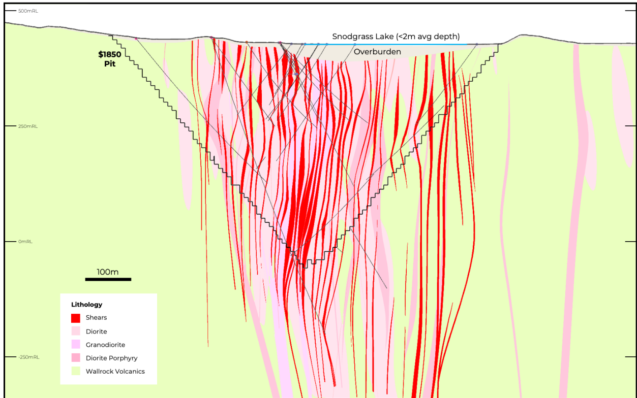
Figure 3: Cross section through the Moss Main Zone showing geology
