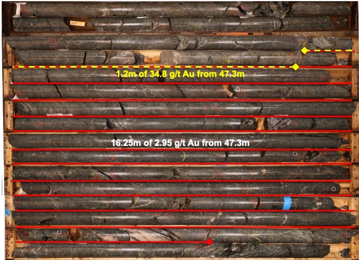
Figure 3: Illustrates drill core from hole MMD-24-133 that is characterized by a stacked sequence of high-grade shears within an altered granodiorite returning 16.25m of 2.95 g/t Au from 47.3-66.55m.
