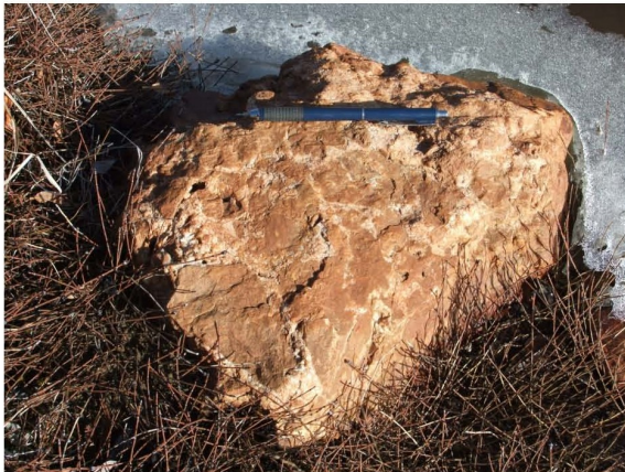
Photo 2: Angular float noted along a small stream near historical placer Au workings, located about 1km north and down slope from rhyolite dome (Photo 1). Sample displays iron-carbonate altered rhyolite breccia cemented with vuggy silica matrix.
