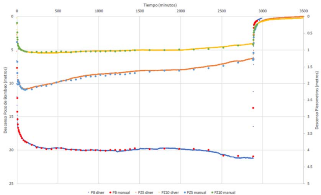
Figure 10-21: Constant Rate 48-h Test result – Well SP-17-14W
