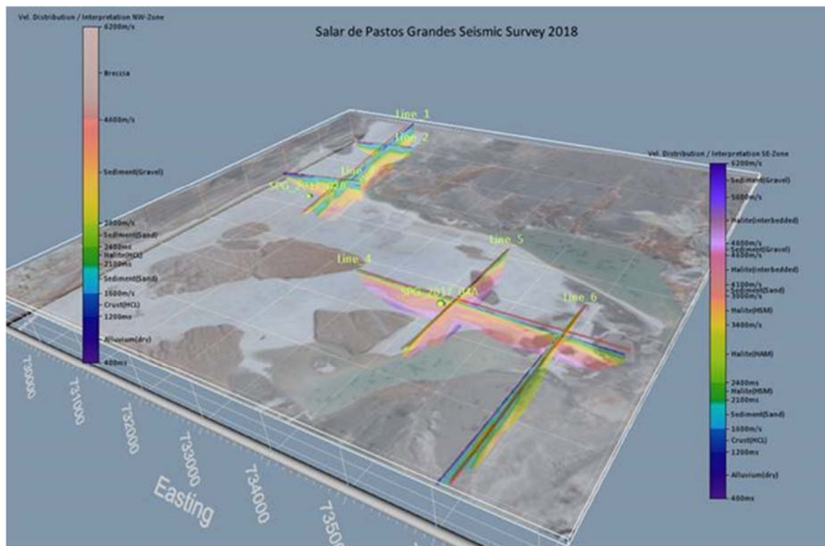
Figure 9-12: Interpreted Seismic Results – Pastos Grandes
