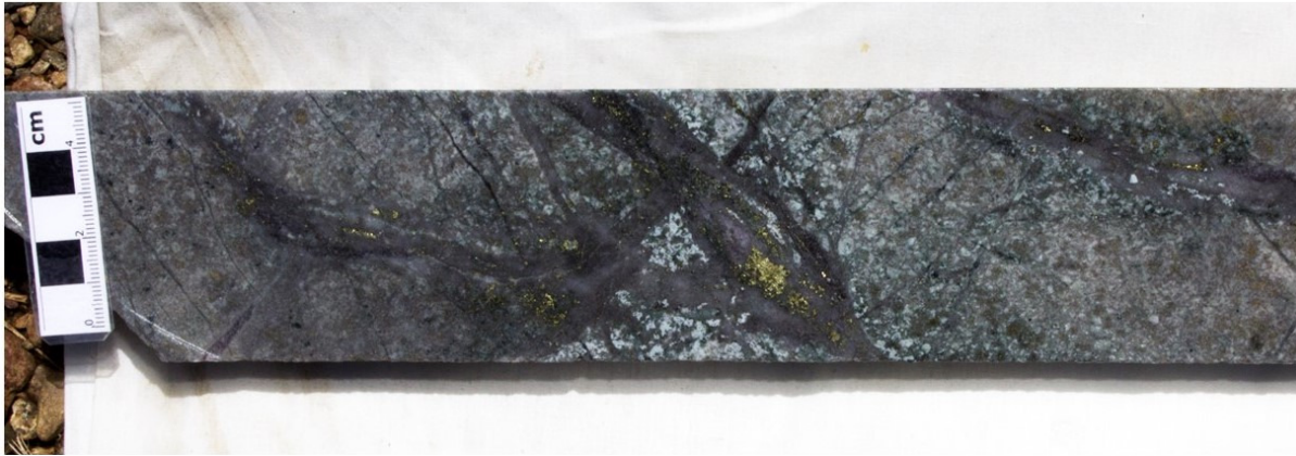
Figure 2. Blue Lake KTDD0001, 413.2m. Classic propylitic porphyry alteration/mineralization. Quartz-chalcopyrite-magnetite B veins amid pervasive chlorite/albite.
