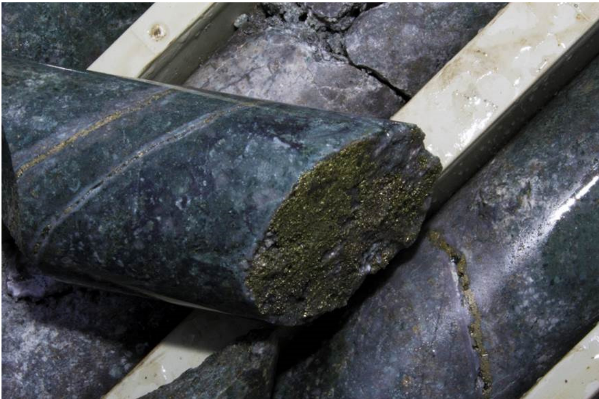
Figure 3. Blue Lake KTDD0006, c. 510m. Quartz-chalcopyrite-magnetite B veins and disseminated chalcopyrite, with pervasive chlorite.
