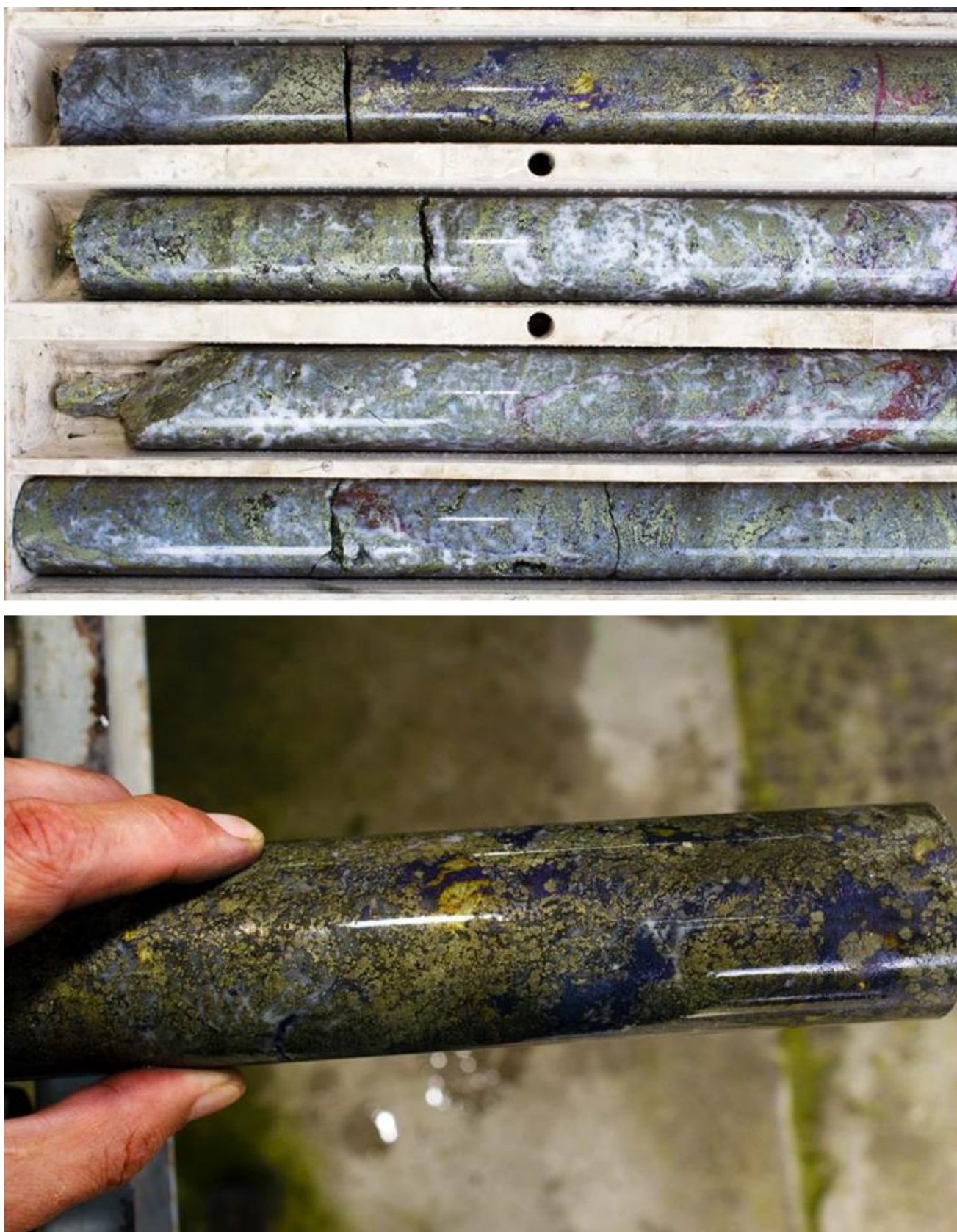
Figure 4 – KMDD0177 Drill Core Intersecting Massive Bornite Mineralization
