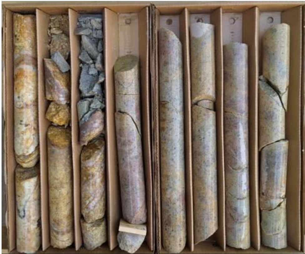
Figure 5: Photo of Drillhole ISB20-11 showing zone of narrow quartz veins from 26.35 m to 31.55 m showing fault breccia contact (lower left) with a potassic-altered leucogranite (right).
