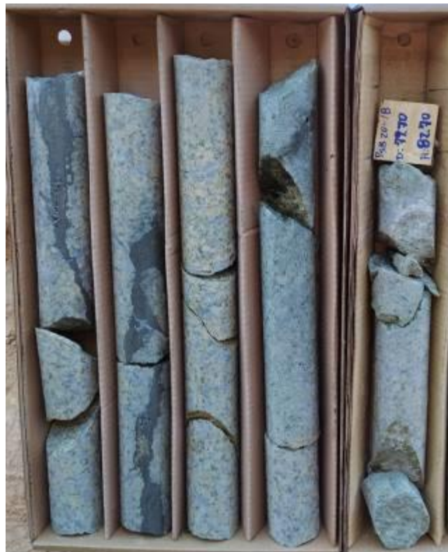
Figure 4: Photo of Drillhole ISB20-18 showing sulphide-rich vein in leucogranite (from 80.5-81.5 m.)
