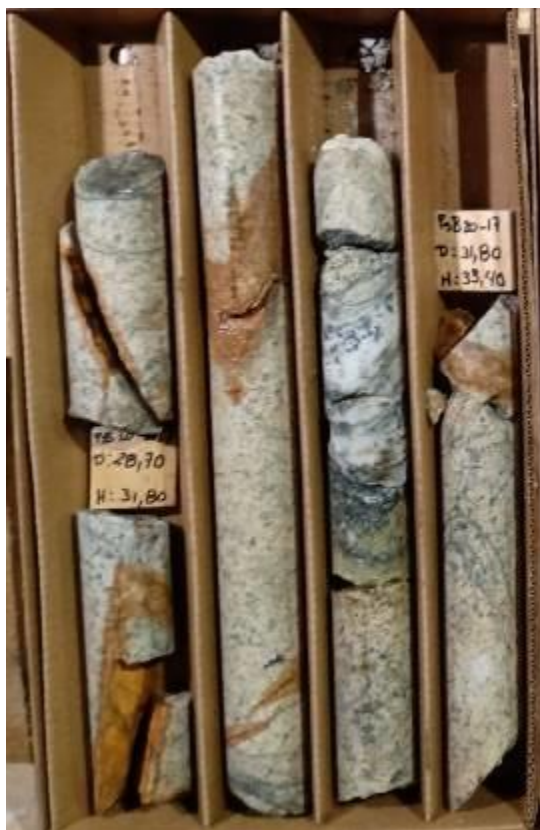
Figure 6: Photo of Drillhole ISB20-17 showing zone of narrow quartz veins from 31.6 m to 33.4 m.
