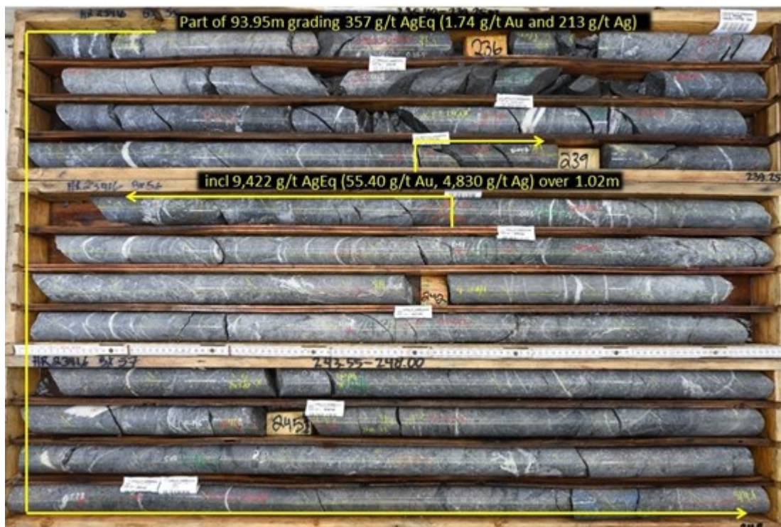
Figure 2. Drill hole HR23-416 from the Homestake Silver deposit. A 12.60-meter section from the 93.95-meter mineralized envelope highlighting the 1.02-meter high-grade multi-pulse vein breccia pathway. Strong alteration and stockwork with local multi-pulse vein and vein breccias can be seen throughout the interval.
