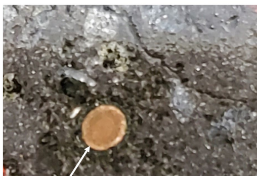
2mm diameter native copper sphere within altered volcanic rock that consists of secondary biotite, feldspar, augite and actinolite alteration minerals.
