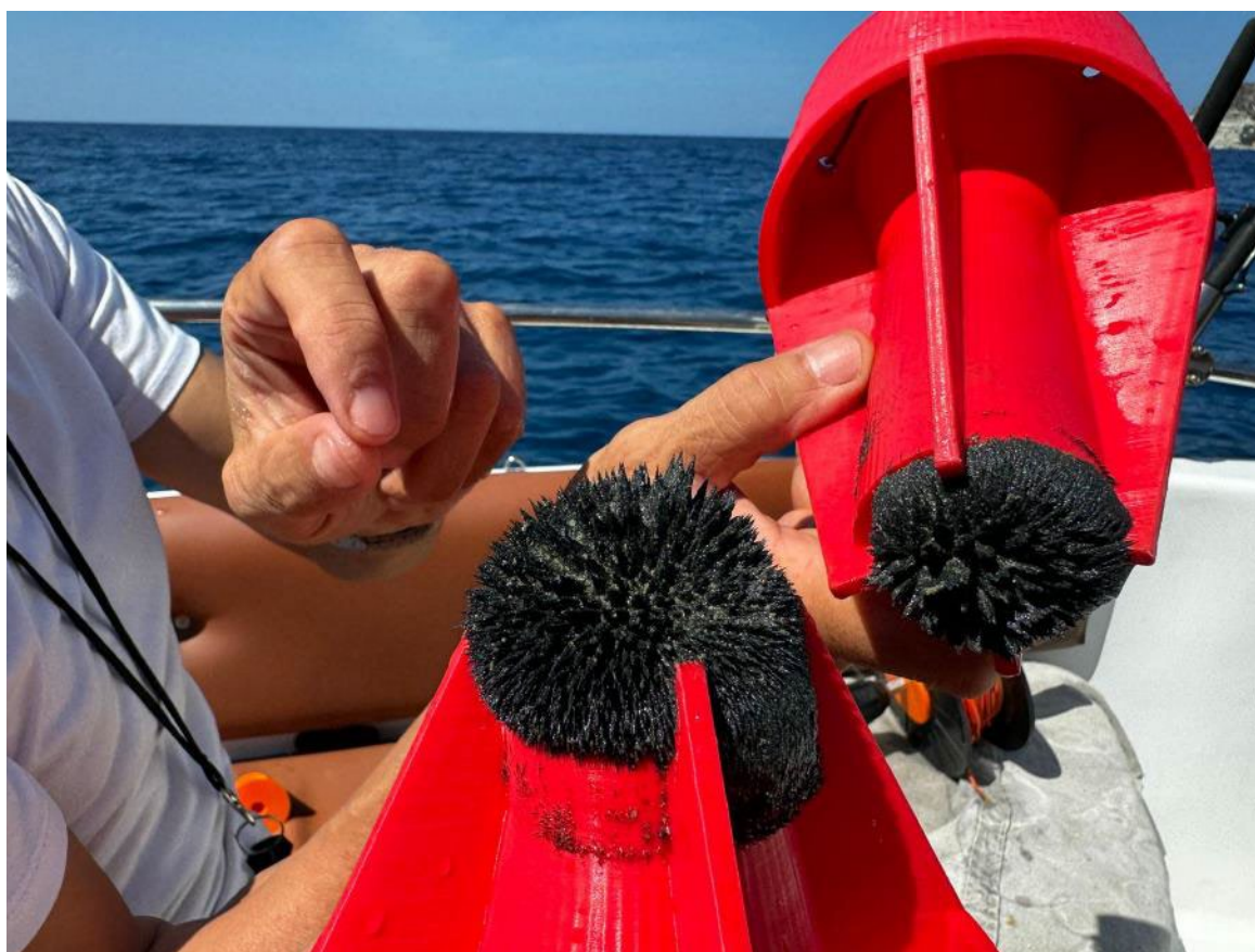
Figure 4: Two rare earth magnet sea probes, both covered in magnetic black sand.
