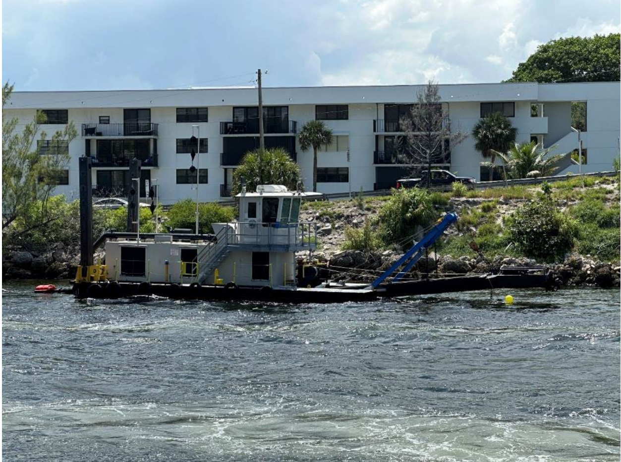
Figure 3: A cutter head suction dredge moored in the channel behind the Rick Rule Conference venue, (Boca Raton, Florida) in July 2024 that Aurania attended. Note that these dredges are used for both civil purposes to clean canals and harbours and for mining alluvials. It operates with a minimum of noise and disturbance and is ideal for clearing channels in proximity to hotels and housing developments.
