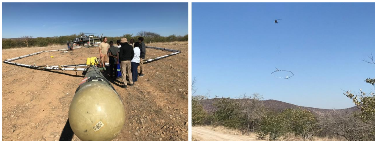
Figure 1 – Namibia Critical Metals geological team being briefed on the SkyTEM system's operation (left). Magnetometer in foreground; EM coil is 28 m in length and 16.5 m wide. System is flown with an AStar 350 helicopter operated by Savannah Helicopters shown flying at Kunene on right.
