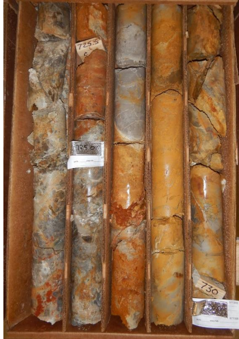
Figure 3 – Photo of oxidized jasperoid breccia from CV22-001, interval 725 - 730 feet (221.0 - 222.5 meters) returned a value of 16.9 g/t Au. To view image please click here
