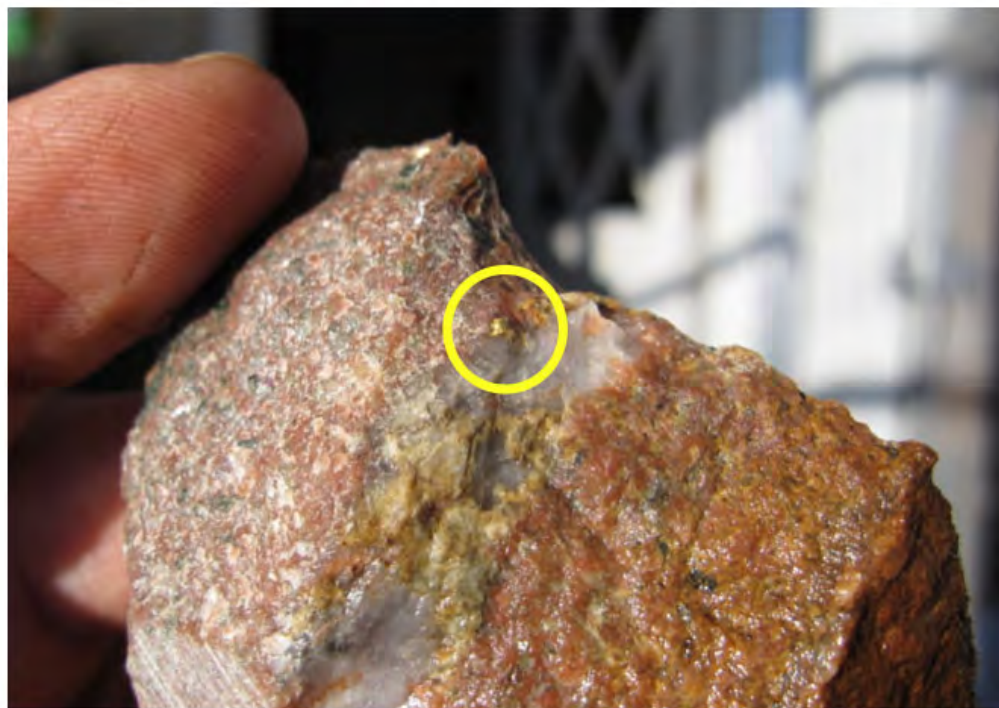
Figure 9. Specimen hosting Visible Gold from Channel Sample I803374
