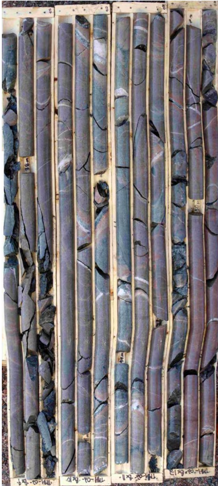
Figure 11: Photo of potassic altered syenite in hole TMH10-02
