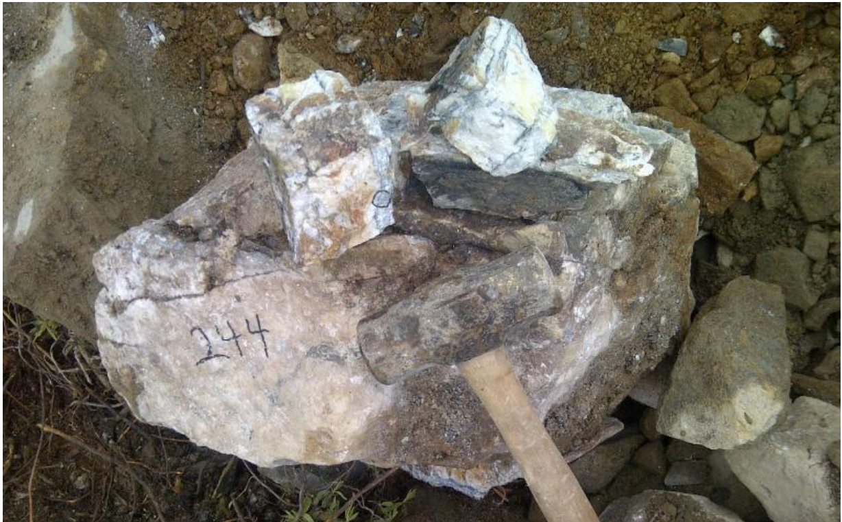
Quartz Vein Boulder with Visible Gold from 2017 Trench 4 (2.9 Kg Grab Sample Returned 332.6 g/t Au)
