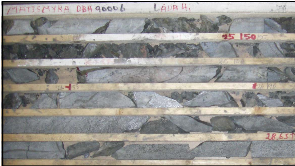
Figure 22: Graphite Mineralization of Drill hole 90006, Mattsmyra deposit, June 2014.
