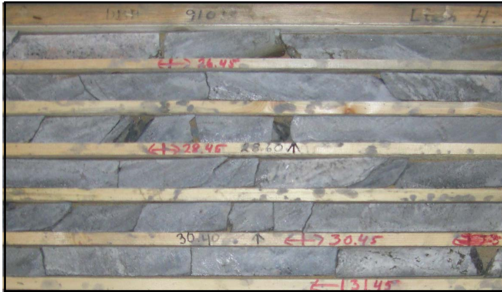
Figure 24: Graphite Mineralization of Drill hole 91013 Gropabo deposit, June 2014
