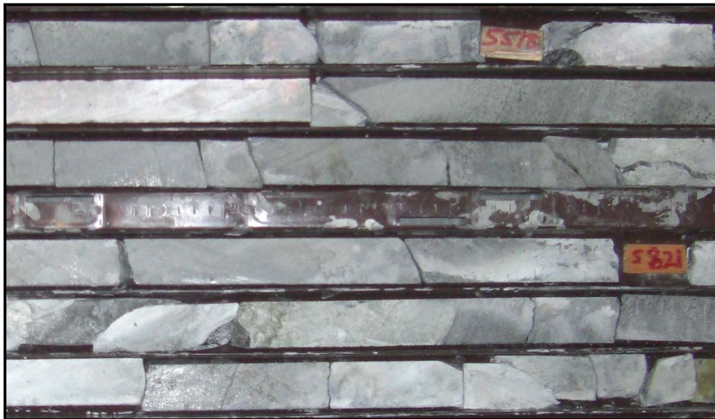
Figure 25: Graphite Mineralization of Drill hole 92003, Gropabo deposit, June 2014
