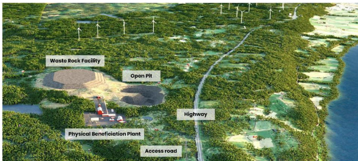
Figure 4 – Main features of the Norra Karr On-site project layout
