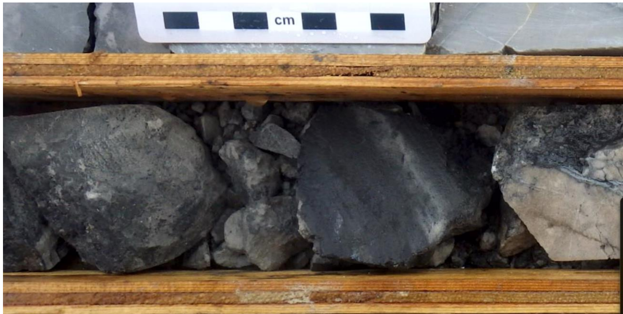
Figure 10: Chalcocite (metallic and dark grey) breccia in drill hole ST23-01 from the 4100N Zone. The interval shown is approximately 58m downhole.
