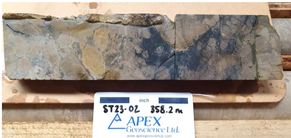
Figure 1: Photo showing example of strong chalcocite (dark grey) breccia fill and veining in drill hole ST23-02 from approximately 358.2m downhole. Chalcocite is a copper sulfide mineral and contains approximately 79.8% copper.
