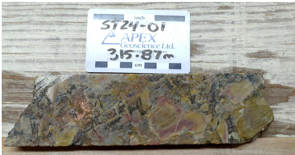
Figure 1: Chalcocite (dark grey) breccia and native copper (metallic) blebs within fractured dolomite in drill hole ST24-01 from approximately 315.87m downhole. This interval yielded 3.7% Cu.
