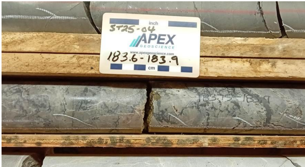
Figure 2: Dense breccia and fracture fill visual pyrite and chalcopyrite from ST25-04 (183.6-183.9m downhole).
