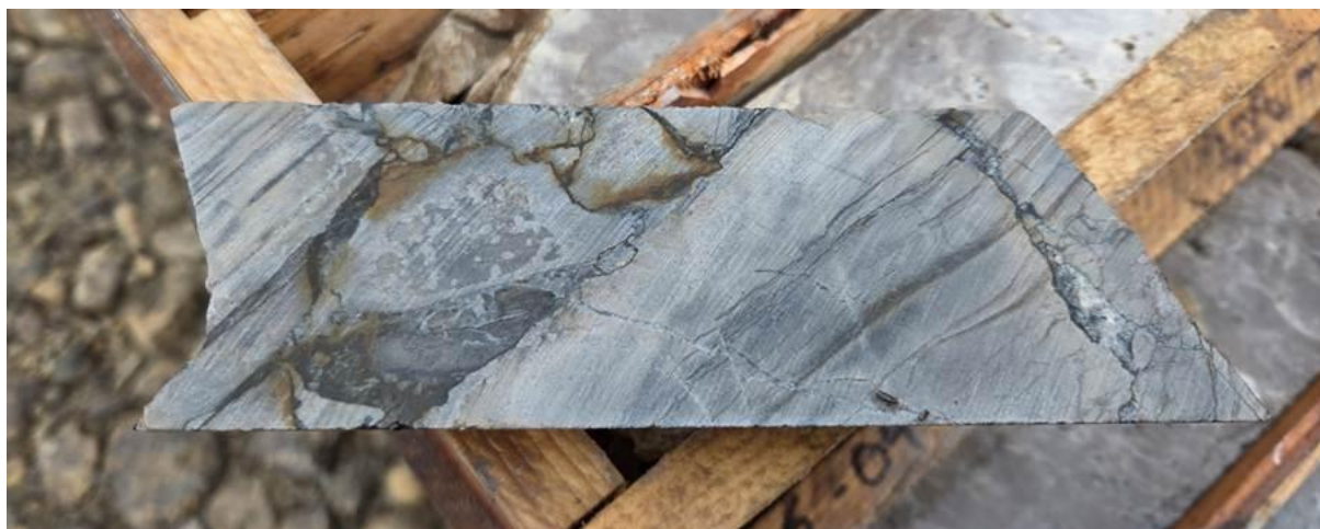
Figure 1: Dense crackle breccia with visual chalcopyrite rimming from drill hole ST25-04 (210.6-210.75m downhole).
