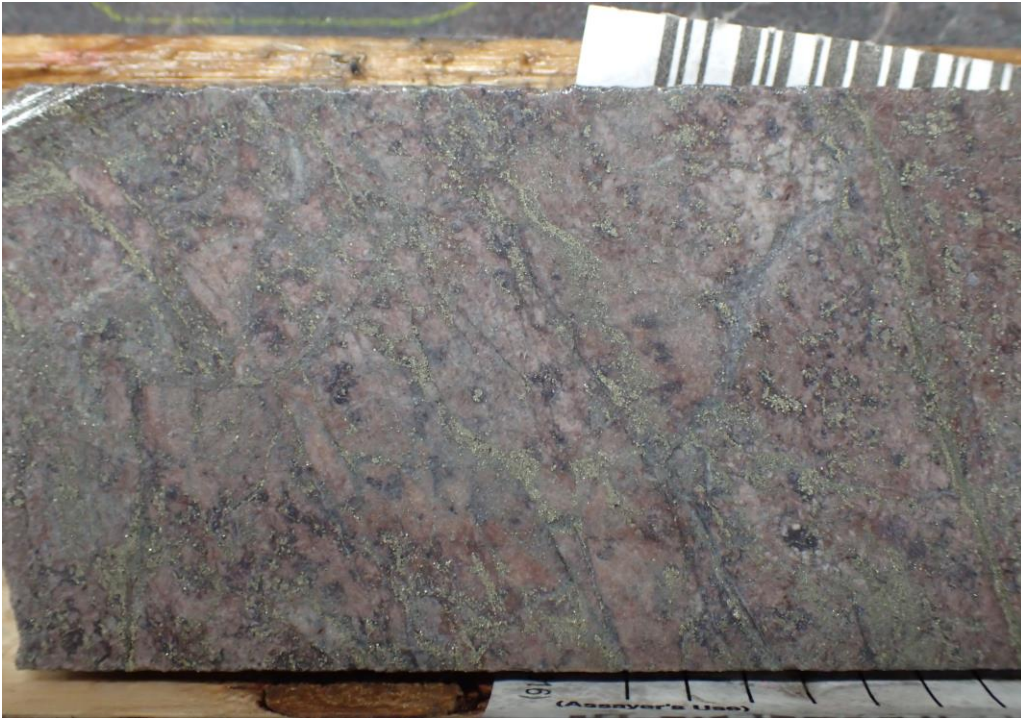
Drill-core Picture 1: (DO-18-218) strongly fractured pink to red syenite with abundant fine pyrite stringers and disseminations.
