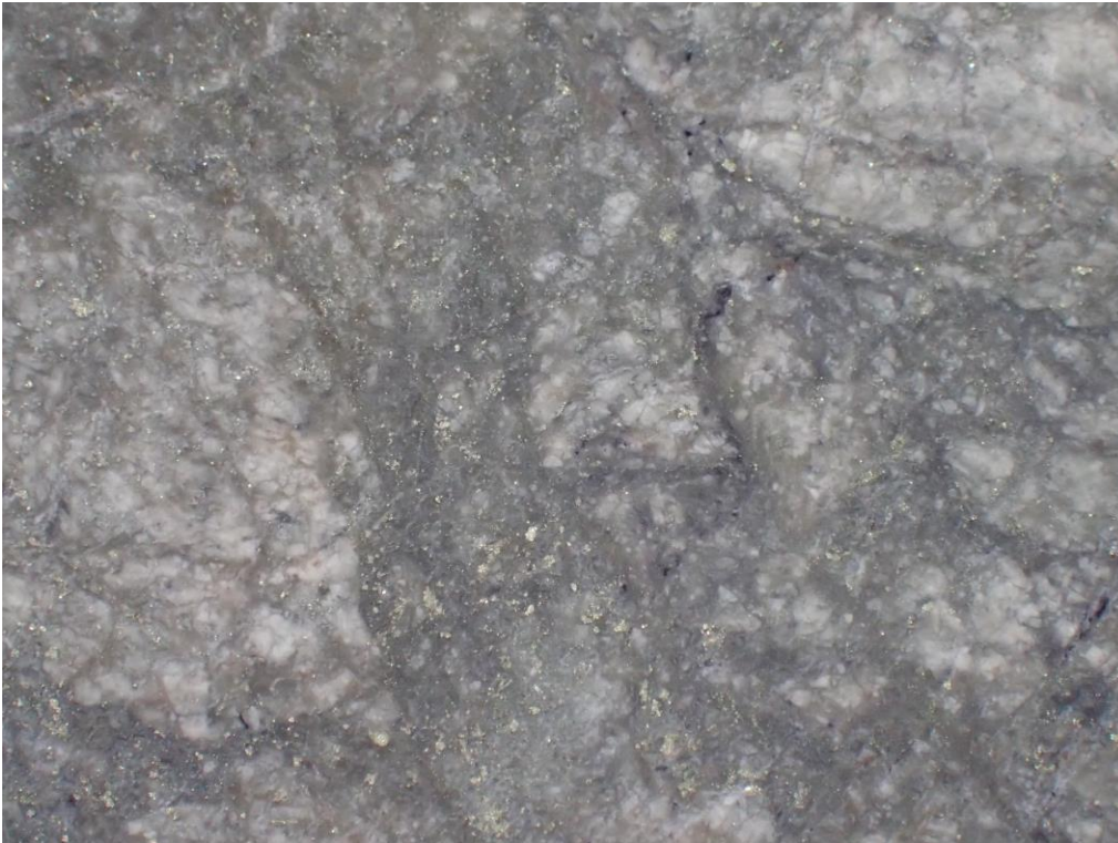
Drill-core Picture 2: (DO-18-218) strongly fractured pale pink syenite with network of pyrite and/or fluorite-filled crackles, with sericitic haloes. Core diameters 47mm.
