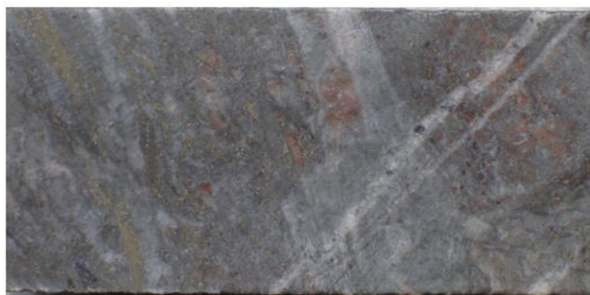
Figure 2: Sample of strongly altered and pyritised basalt with syenite fragments in interval grading 9.74 g/t Au; field of view 47.6mm.
