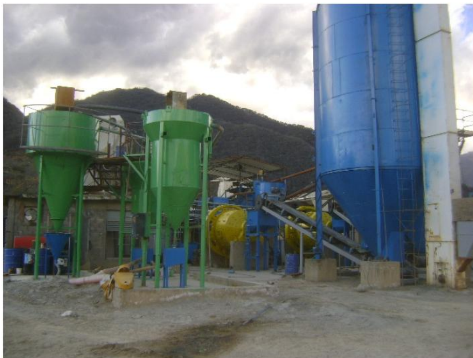
Figure 13.5. (Right to left) Fine ore bin and bucket elevator, belt conveyor 5a, Hardinge ball mills (yellow), and SEDCON final tailings thickeners (green).
