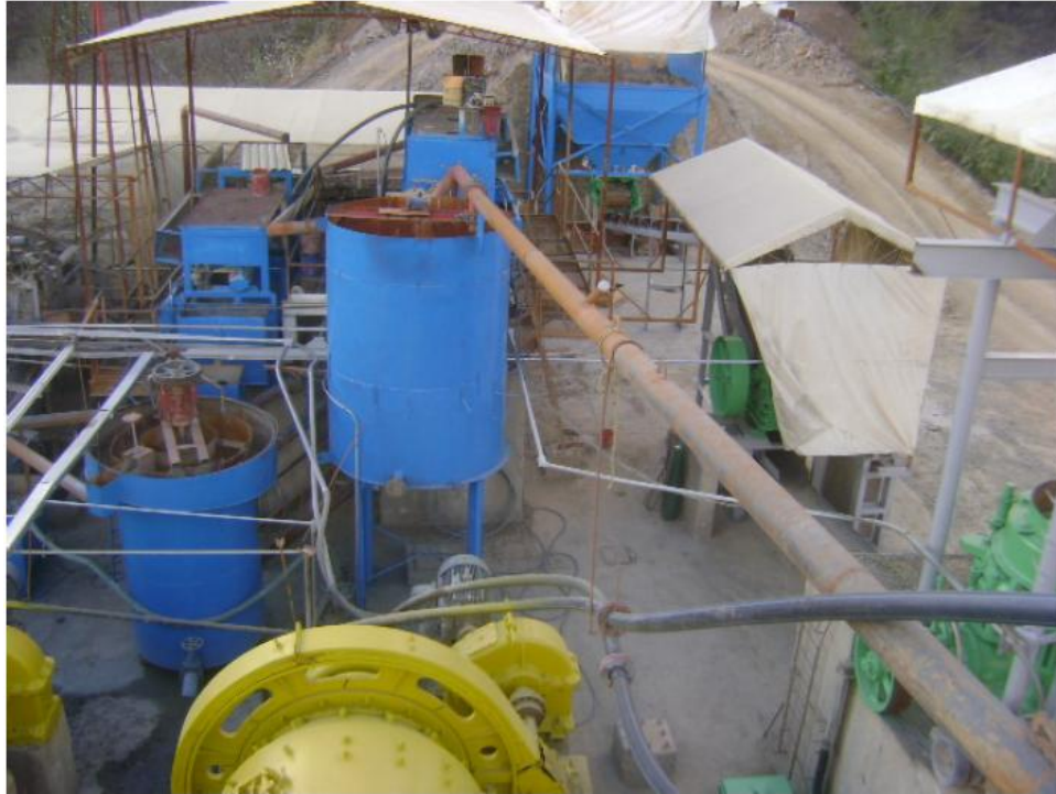
Figure 13.7. From left to right (in blue): cylindrical scavenger flotation cell, slurry conditioning tank, and rougher flotation banks.
