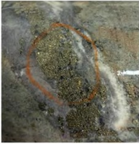
PE-26-030: 5 specs of visible gold 183.35 m in Py
