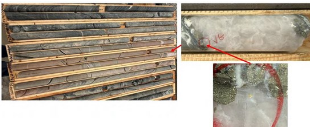
220.60 - 220.75 metres: Single spec of visible gold and coarse pyrite observed in NQ drill core sample, hosted in a quartz-ankerite extensional vein.
