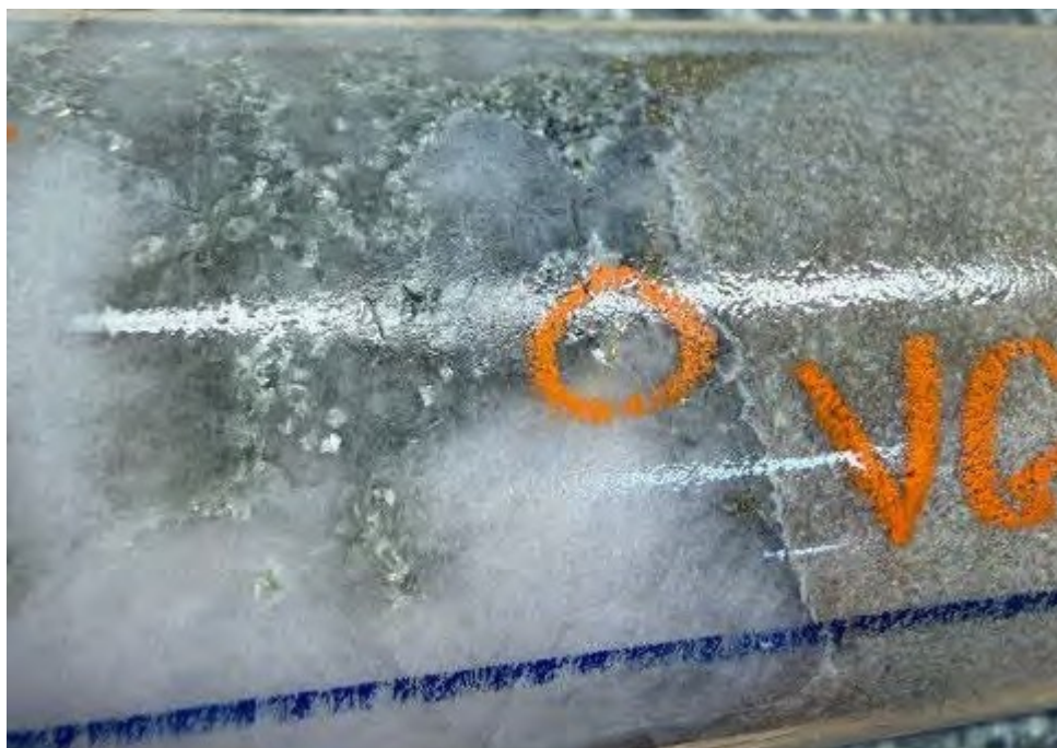
178.0 metres: Visible gold intersection observed in NQ drill core sample.
