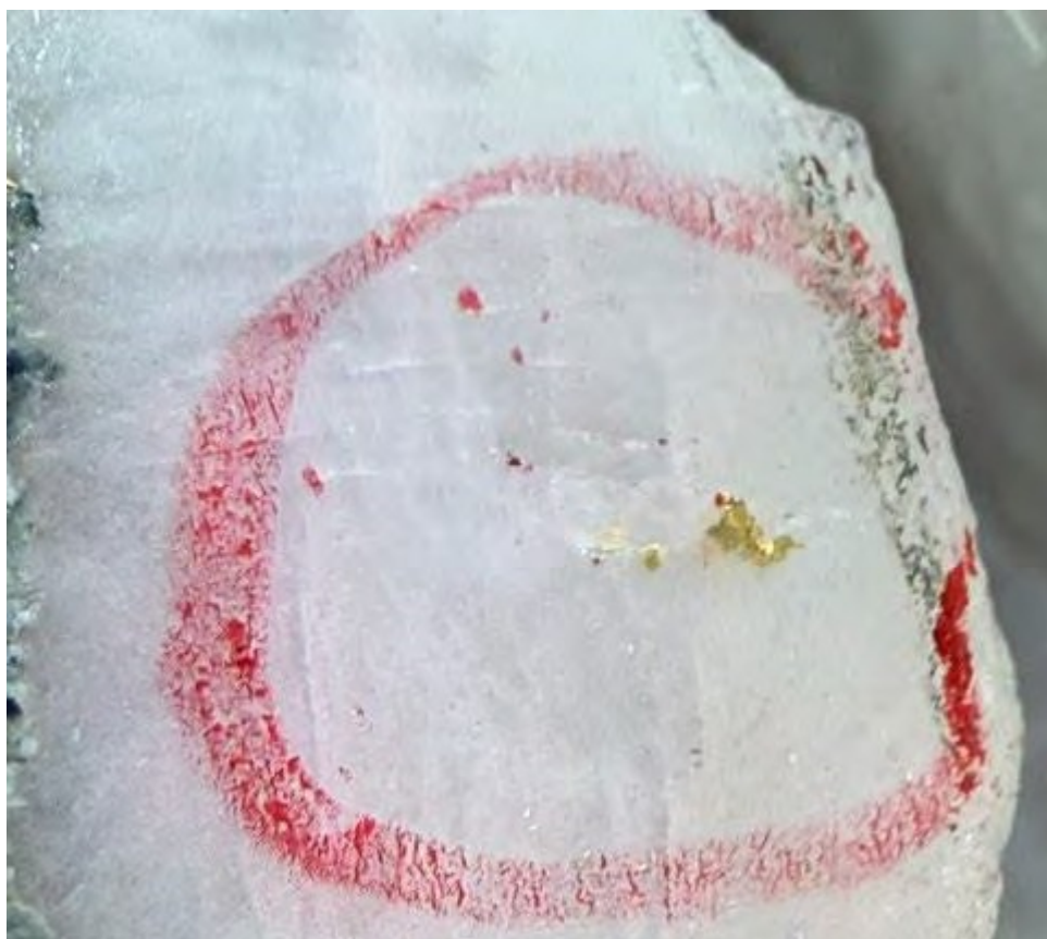
328.70 metres: Visible gold intersection observed in NQ drill core sample.
