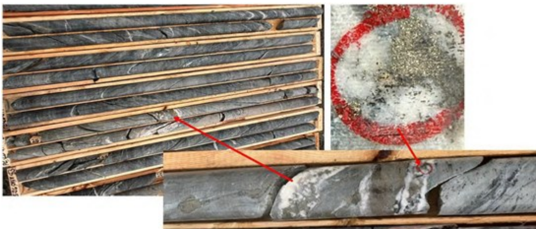
252.40 - 252.55 metres: Single spec of visible gold and coarse pyrite observed in NQ drill core sample, hosted in a quartz-ankerite-chlorite extensional vein.
