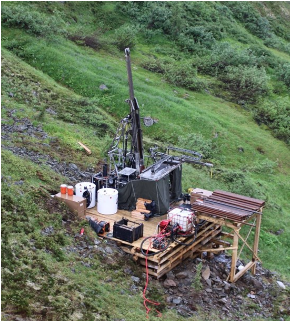
SUN23-002: Major Drilling EF75 setup and drilling at Sun23-002.
