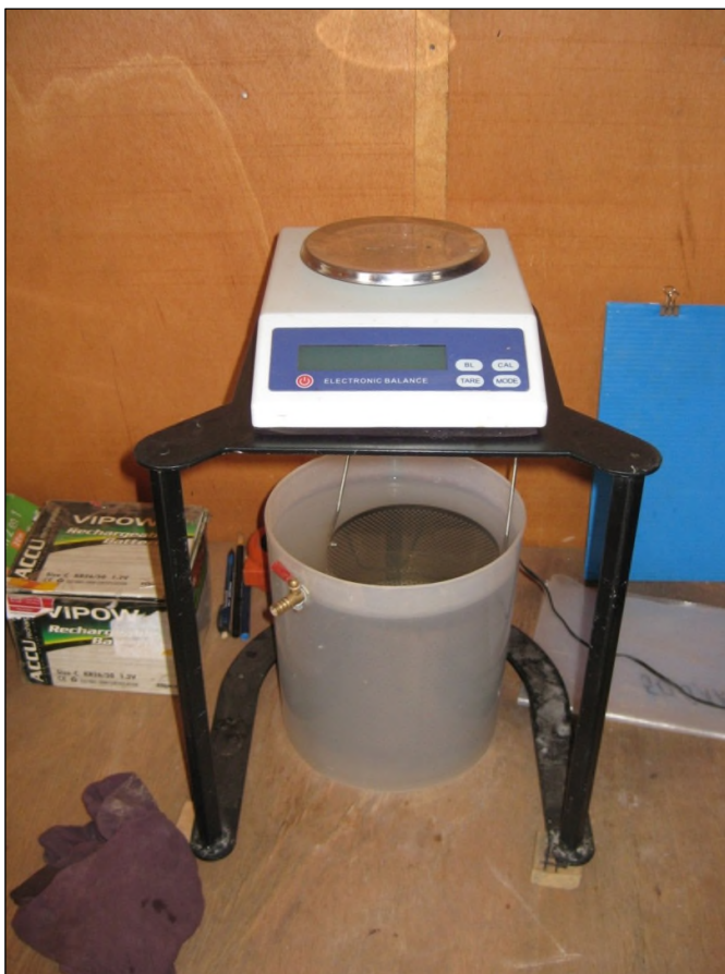
Figure 10-5 Density Measurement Equipment
