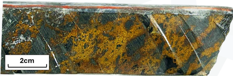
TDH09 1.5 metres at 6.40 % Cu from 205.8 metres 1 chalcopyrite (copper sulphide) in chlorite-magnetite-quartz altered intermediate volcanoclastic breccia. Chalcopyrite tarnished by length of time in core tray
