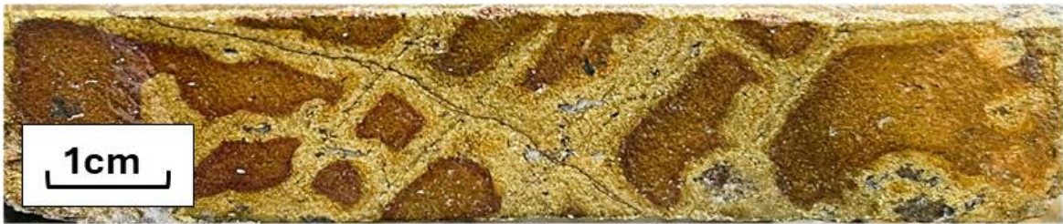
Figure 3 – Photo of diamond core completed by Australian Oil & Gas Minerals Pty Ltd (1970's). Sample interval of 4.6 metres at 18.54 % Cu from 57.9 metres in TDH01 containing massive chalcopyrite (copper sulphide). Core diameter is BQ (36.4mm) with quarter core retained as a representative sample. Chalcopyrite is tarnished brown by length of time in core tray.
