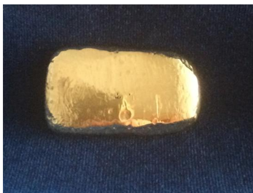
64 grams of gold recovered by gravimetric method
