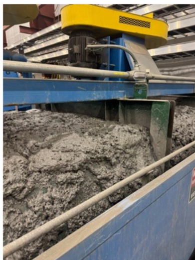
Lead Concentrate being floated in flotation circuit
