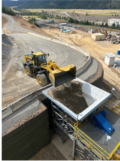
Ore loading into crusher hopper
