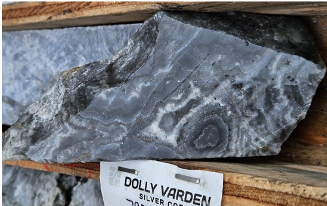
Figure 4. Cut core sample face of Wolf Vein silver mineralization in DV24-412 @ 792.10m consisting of disseminated native silver (red arrows) and argentite (black bands) in epithermal grey silica vein with colloform texture open space fill. From an individual sample length of 0.62 meters grading 929 g/t Ag .
