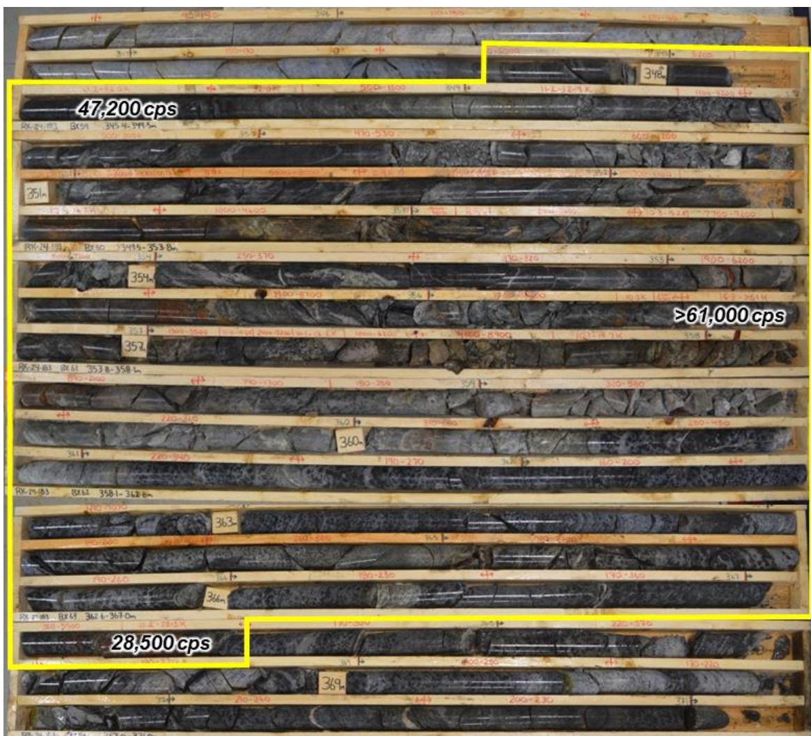
Figure 4: Localized basement-hosted uranium mineralization between 347.7 and 367.5 m (outlined in yellow)
