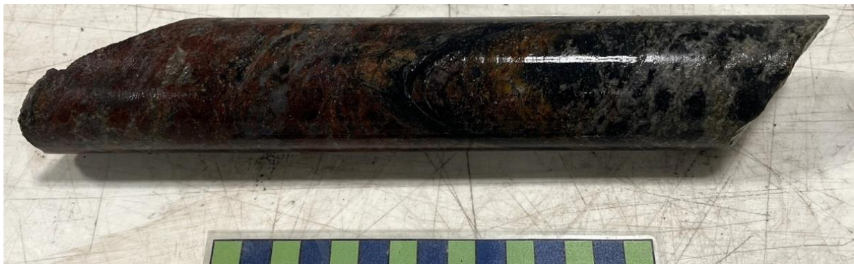
Figure 7: Secondary mineralization along microfractures and foliation at 367.3 m, maximum peak of 28,500 cps
