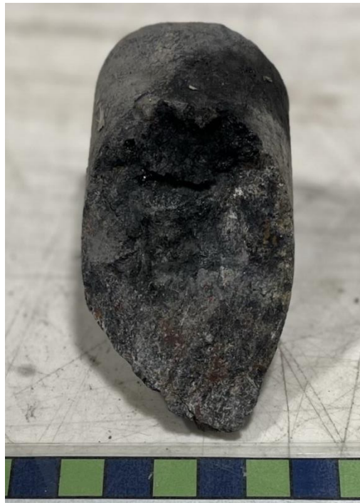
Figure 6: Semi-massive, primary uranium mineralization hosted in competent garnetiferous orthogneiss at 356.9 m, maximum peak of >61,000 cps
