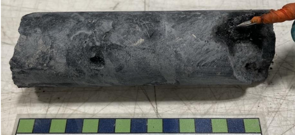
Figure 5: Semi-massive, primary uranium mineralization at 348.5 m, maximum peak of 47,200 cps as shown
