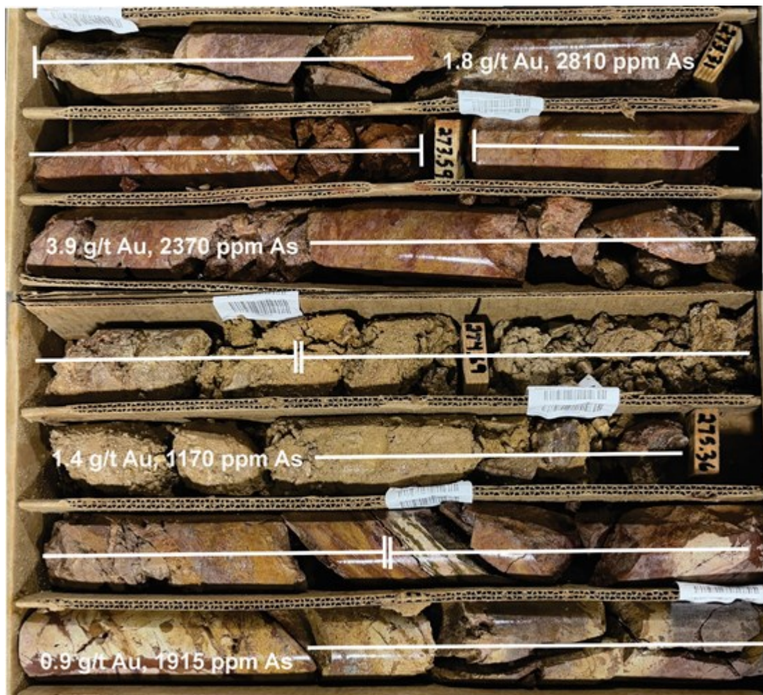
Figure 5. Gold and Arsenic-enriched drill core from HSC002.
