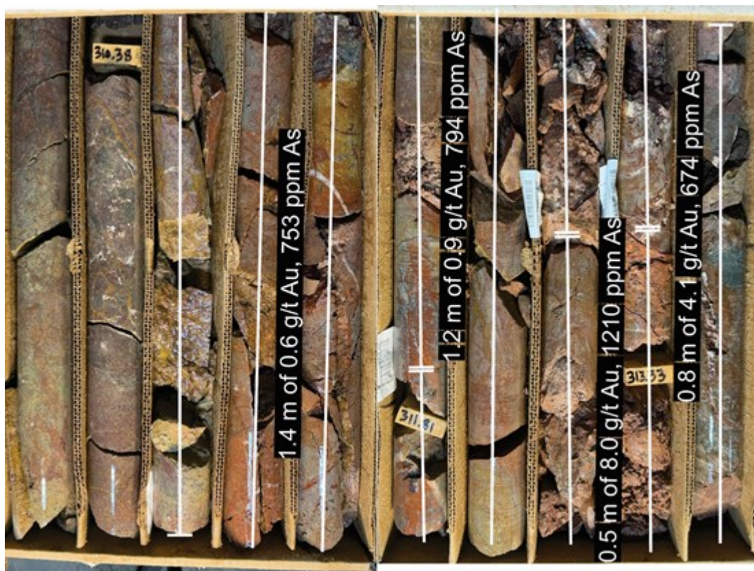
Figure 5. Gold and Arsenic-enriched drill core from HSC-002. The composite intercept is 3.9 m of 2.4 g/t gold and 807 ppm arsenic starting at 310.4 meters hole depth.
