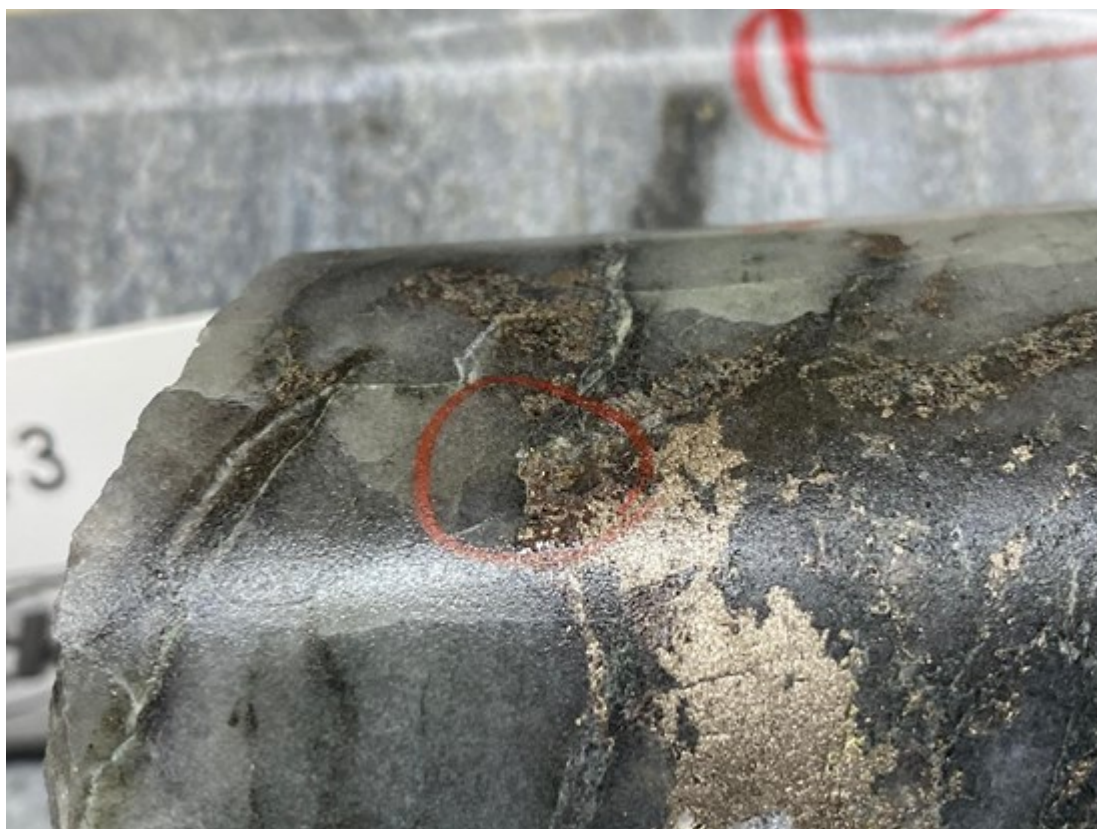
Figure 3: Visible gold associated with quartz-pyrrhotite-chalcopyrite and sphalerite vein into a mineralised and strongly altered mylonite -Hole EM21-167 (4 grains 1mm in circle)
