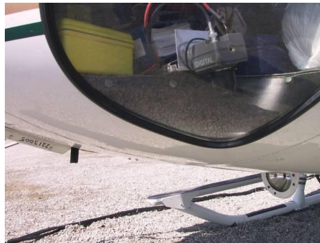
Figure 4. Digital video camera typical mounting location
