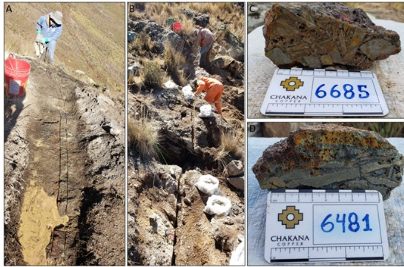
Figure 3 - photos showing channel sampling technique and examples of channel samples: A) channel cut into outcrop with diamond saw, channel width is 7.5 cm; B) channel samples are chiseled from outcrop and transferred to sample bags for each specified sample interval; C-D) examples of breccia samples from channel sampling program.
