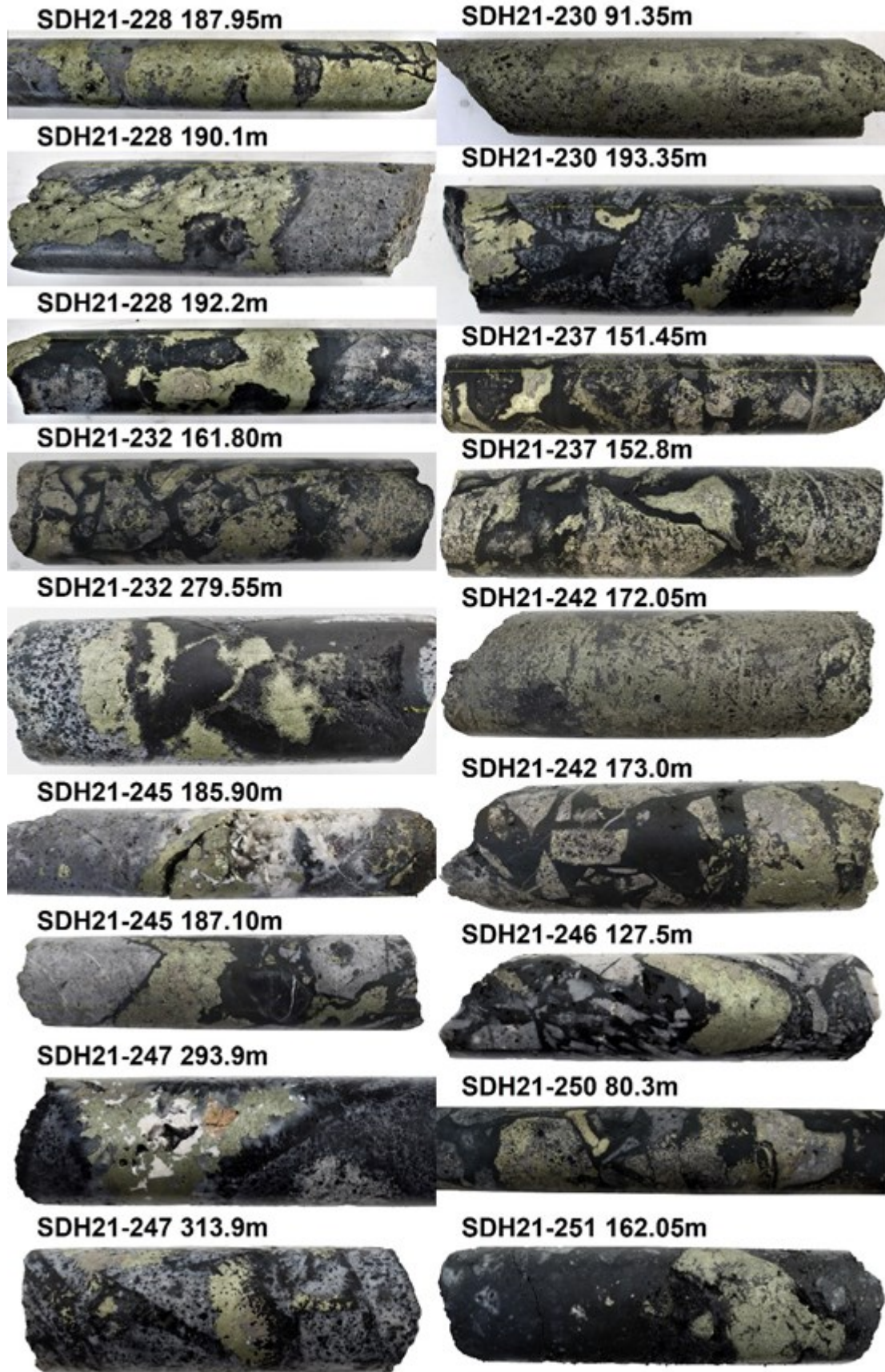
Figure 4 - Select core photos from Huancarama reported in this release: SDH21-228 (187.95m) semi-massive chalcopyrite-pyrite replacement of tourmaline breccia; SDH21-228 (190.1m) chalcopyrite filling open cavity in breccia; SDH21-228 (192.2m) chalcopyrite-tourmaline-cemented breccia; SDH21-230 (91.35m) massive chalcopyrite; SDH21-230 (193.35m) chalcopyrite-tourmaline-cemented breccia; SDH21-232 (161.80m) chalcopyrite-pyrite replacement of clasts; SDH21-232 (279.55m) chalcopyrite-tourmaline-cemented breccia; SDH21-237 (151.45m) chalcopyrite-tourmaline-cemented breccia and
