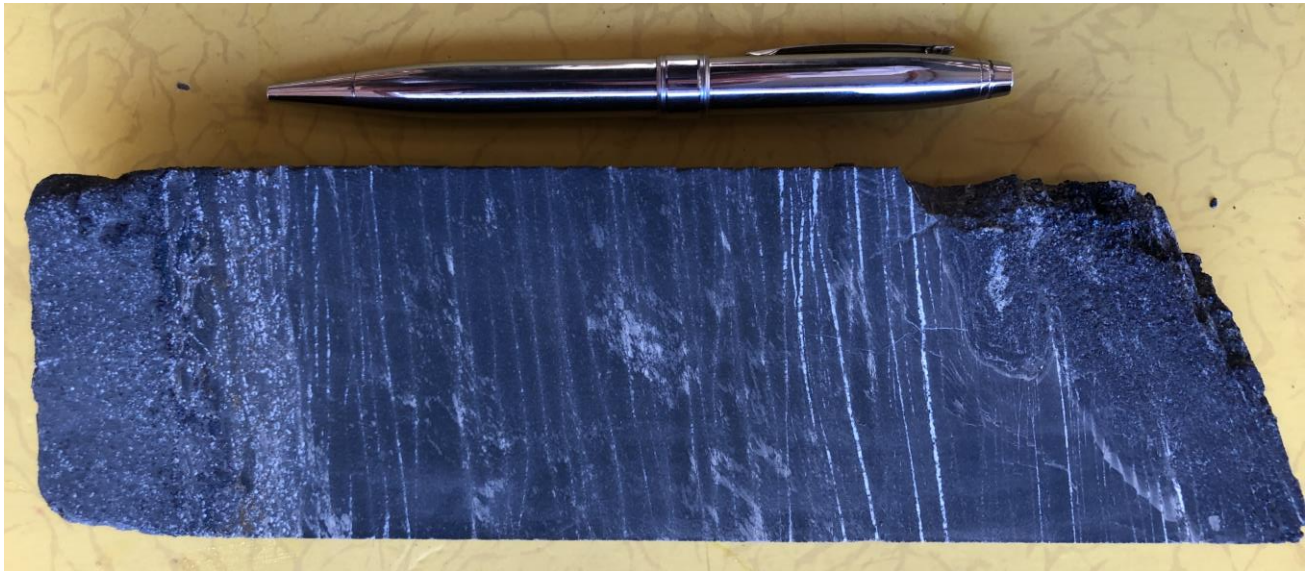
Figure 9: Very strong chalcopyrite mineralization in siltstone from a depth of 221.8 metres in new hole DD1524. Assays are pending for this high-grade hole, which currently is defining the western limit of the 350-metre drill tested zone.
