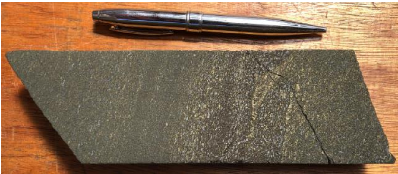
Figure 9: Very strong chalcopyrite mineralization in siltstone from a depth of 221.8 metres in new hole DD1524. Assays are pending for this high-grade hole, which currently is defining the western limit of the 350-metre drill tested zone.
