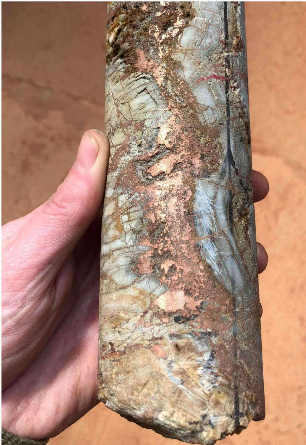
Figure 5: Core from hole DD1571 at a depth of 214 metres, showing disseminated chalcocite with a wide vein of native copper cutting through it in the breccia zone.
